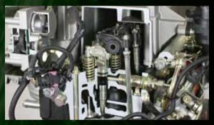
The modern DEUTZ engines, compliant with the III B (Tier 4 Interim) standard, have four valves per cylinder, Common Rail system and after treatment of exhaust emissions with SCR. A formidable combination that allows the engine to provide maximum performance under any conditions. Thanks to the SCR converter, which replaces the conventional exhaust gas recirculation system, the engine works with optimal efficiency and performance.
