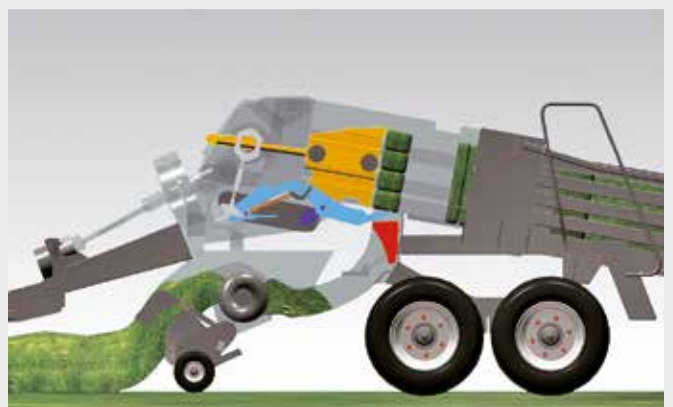
4. Once the measuring plate is pushed back, it activates the second function of the feeder fork system. The fork makes a different movement that empties the pre-chamber and pushes the perfectly formed flake into the bale chamber.
