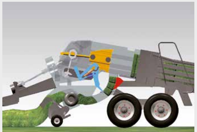
3. The single-acting feeder fork continues to form the bale flake until the measuring plate (red) is pushed back with a predetermined force.
