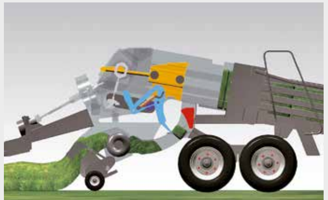
2. The feeder fork (blue) provides an active filling of the pre-chamber.
