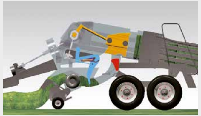
1. The INTEGRAL ROTOR actively delivers the crop to the chamber.
