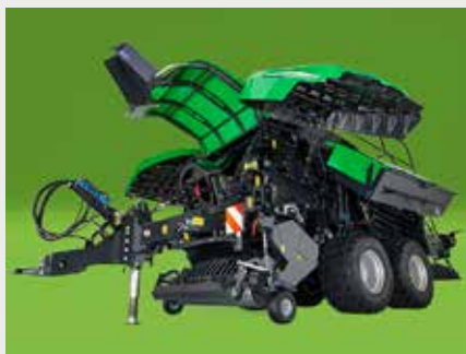
↑ The twine boxes swing out completely for easy access to the vital parts of the machine. Behind the full-access side doors, 32 x 13 kg spools of twine can be stored.
