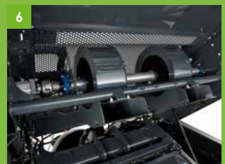
Knotter cleaning turbines
