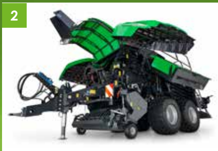
Pivoting twine boxes for easy maintenance
