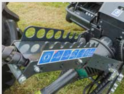
↑ For clean and tidy storage, the balers are equipped with a convenient storage place for the hoses and cables needed to operate the machine.
