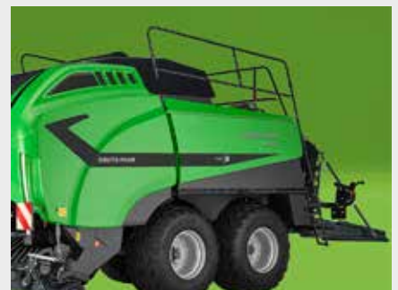
↑ For more safety, the knotted deck is equipped with solid stairs and a safety railing. The safety railing can be folded down easily to reduce the height of the machine during transport.
