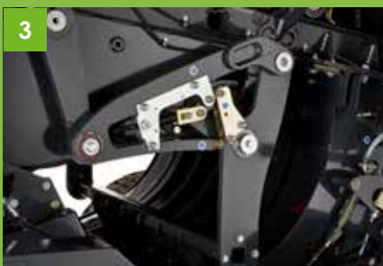
POWER DENSITY pre-chamber system
