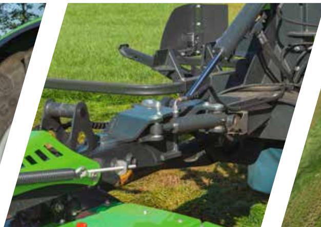
> LIFT-CONTROL hydraulische obstakelbeveiliging.
