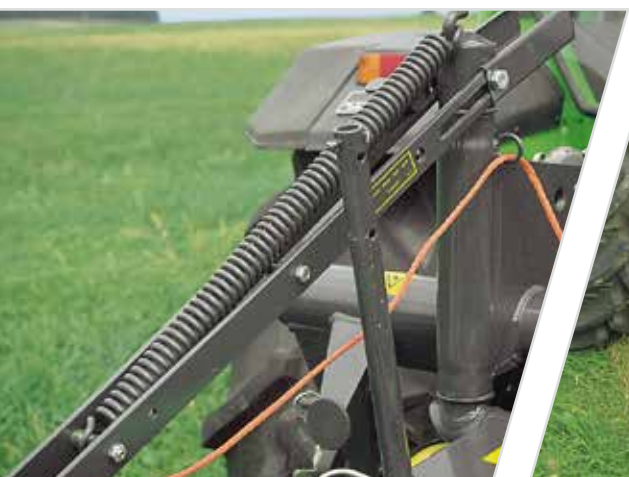
> The compensation springs keep ground pressure low.
