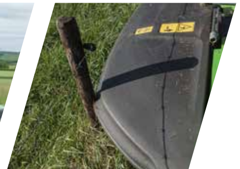
3 Redesigned and patented* FLEXPROTECT flexible side cover.
