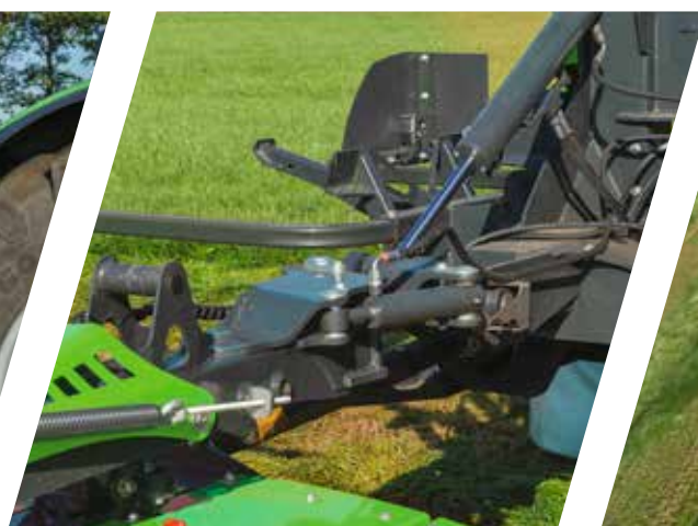
> LIFT-CONTROL hydraulic safety break back system.
