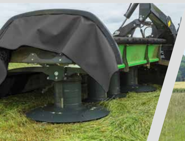
> Easy access and cleaning thanks to the foldable side guards.
