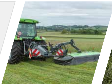
2 Headstock with trailed linkage geometry.
