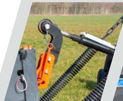
> FLEXTOP flexible top link connection (only in combination with a fixed headstock).
