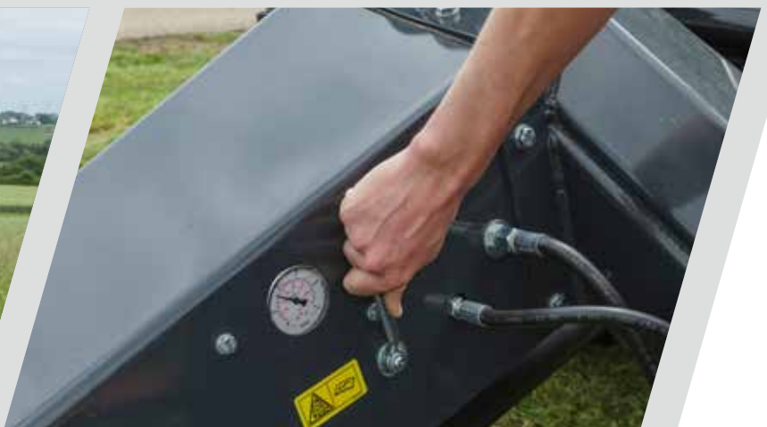
> LIFT-CONTROL hydro-pneumatic suspension system.
