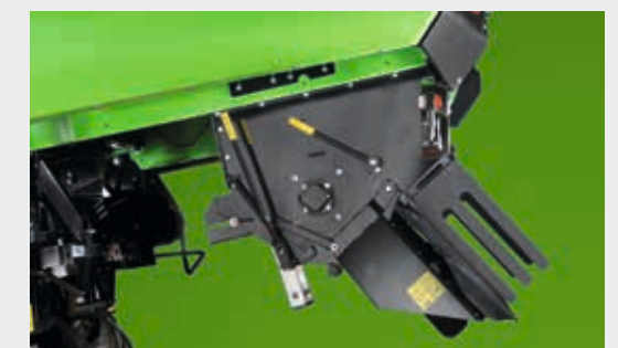
Straw-chopper unit with spreader adjustable in 3 positions. The spreader unit is converted to a chute for the long straw while not in use.
