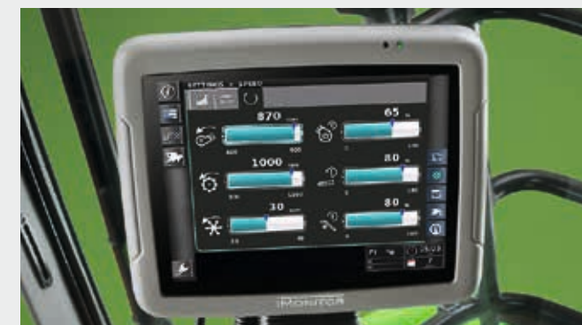
➤ All combine parameters and functions are managed directly on the iMonitor.
