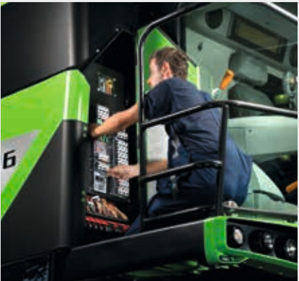
↑ Easy access to the fuse box.
