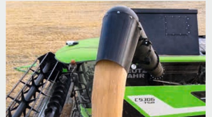
Integrated light and camera on the unloading pipe to check the unloading operations.
