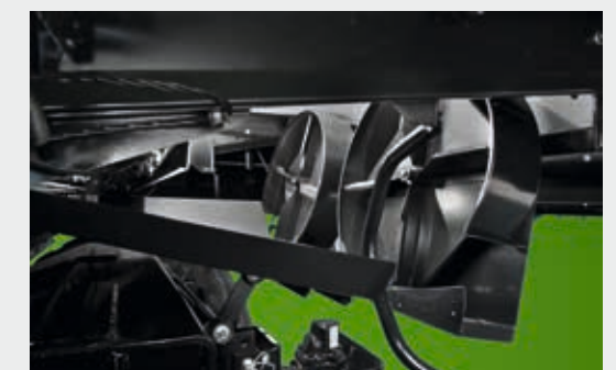
The spread of the chopped straw covering the entire width of the cutting header in all conditions. Integrated chaff spreader for an even preparation of the soil.
