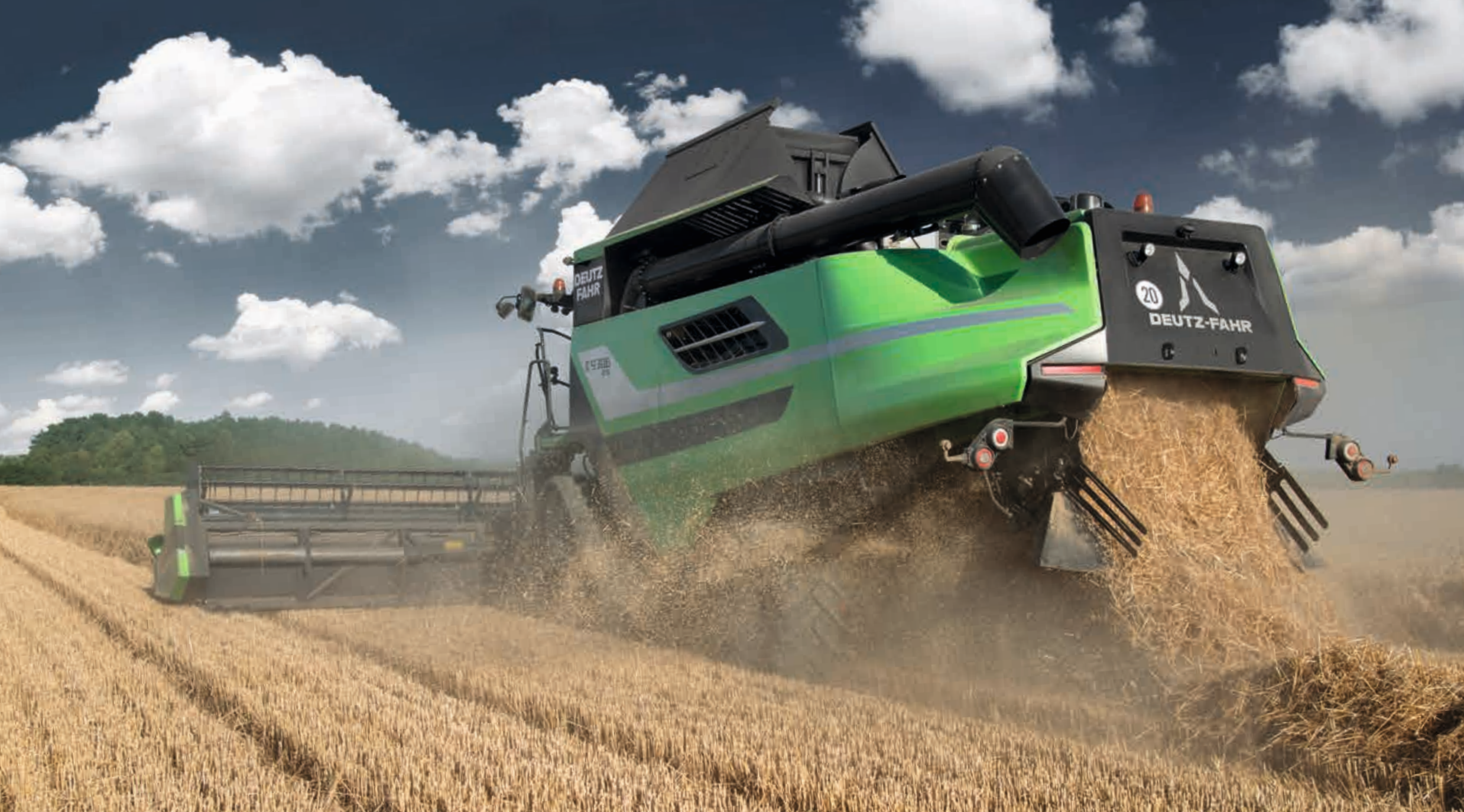
Big straw-hood discharge chute to maximize the product flow of the long straw.
