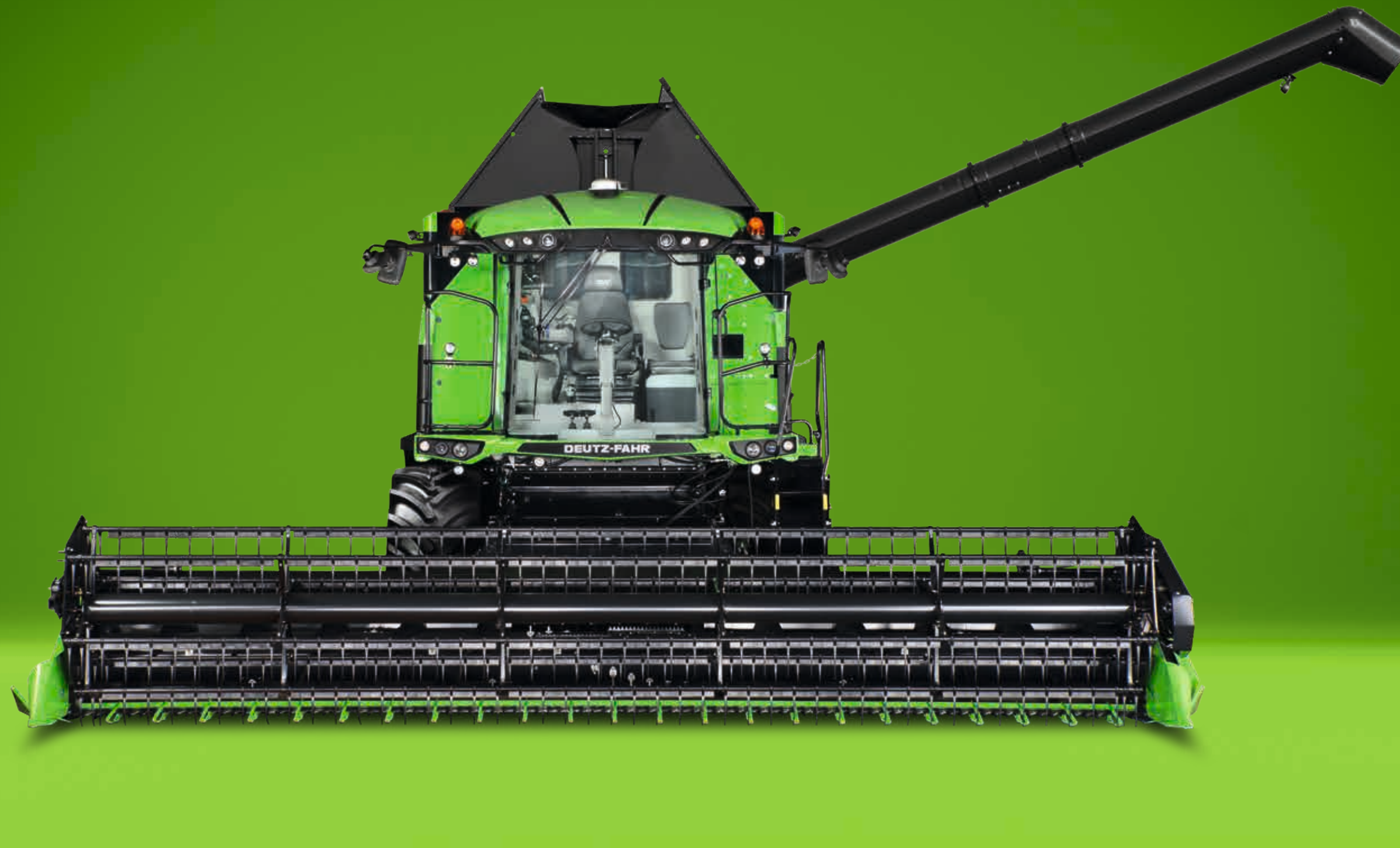
↑ The SCHUMACHER EASY CUT II system: cutting rate of 1220 strokes per minute but reduced wear and power absorption.
