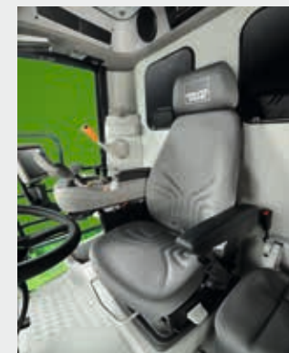
Dual inspection window in the cabin, easy sample pick up tray just outside the cabin.
