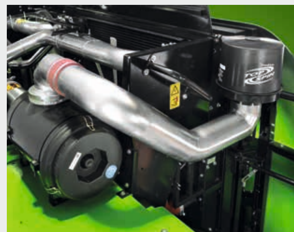
↑ Pre-cleaning engine air filter with automatic self-cleaning system.
