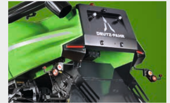
Big straw-hood discharge chute to maximize the product flow of the long straw.
