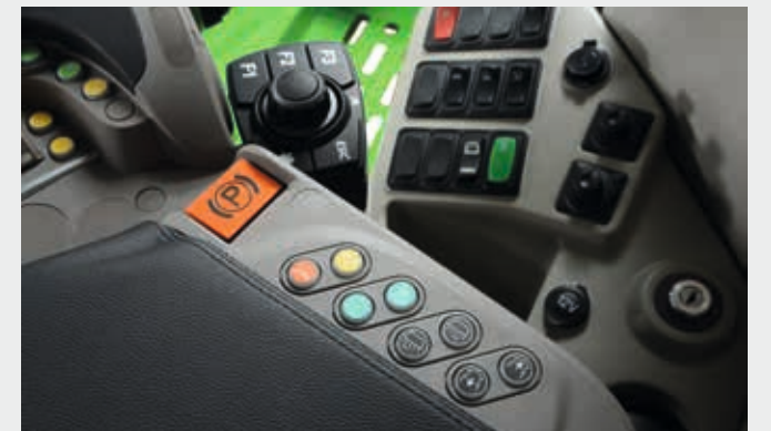
➤ At the rear of the armrest are the controls for 4wd, park brake, grain tank opening, MMI and the new dashboard with USB outlets.
