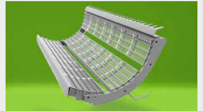
Segmented concave to easily adapt the combine to different crop or different harvesting conditions with spacing between the wires available from 11 mm to 20 mm.
