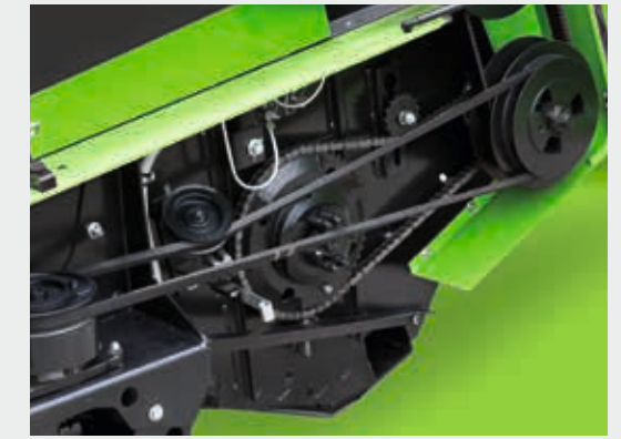
↑ The SCHUMACHER EASY CUT II system: cutting rate of 1220 strokes per minute but reduced wear and power absorption.
