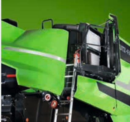
↑ Full access to the radiators: wide opening and dedicated platform.
