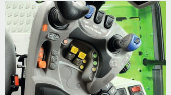
➤ Easy selection of the combine systems - concave (front and rear), sieves (upper or lower) and Turbo - separator with easy adjustment via 3 touch buttons. Header controls for mode, height and soil pressure adjustment. Joystick control for the BALANCE system provides intuitive and accurate adjustment.
