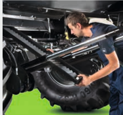
↑ The segments of the preparation pan are easily extracted from the stone trap.
