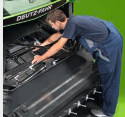
↑ Easy access to adjust and check the chains on the feeder channel.
