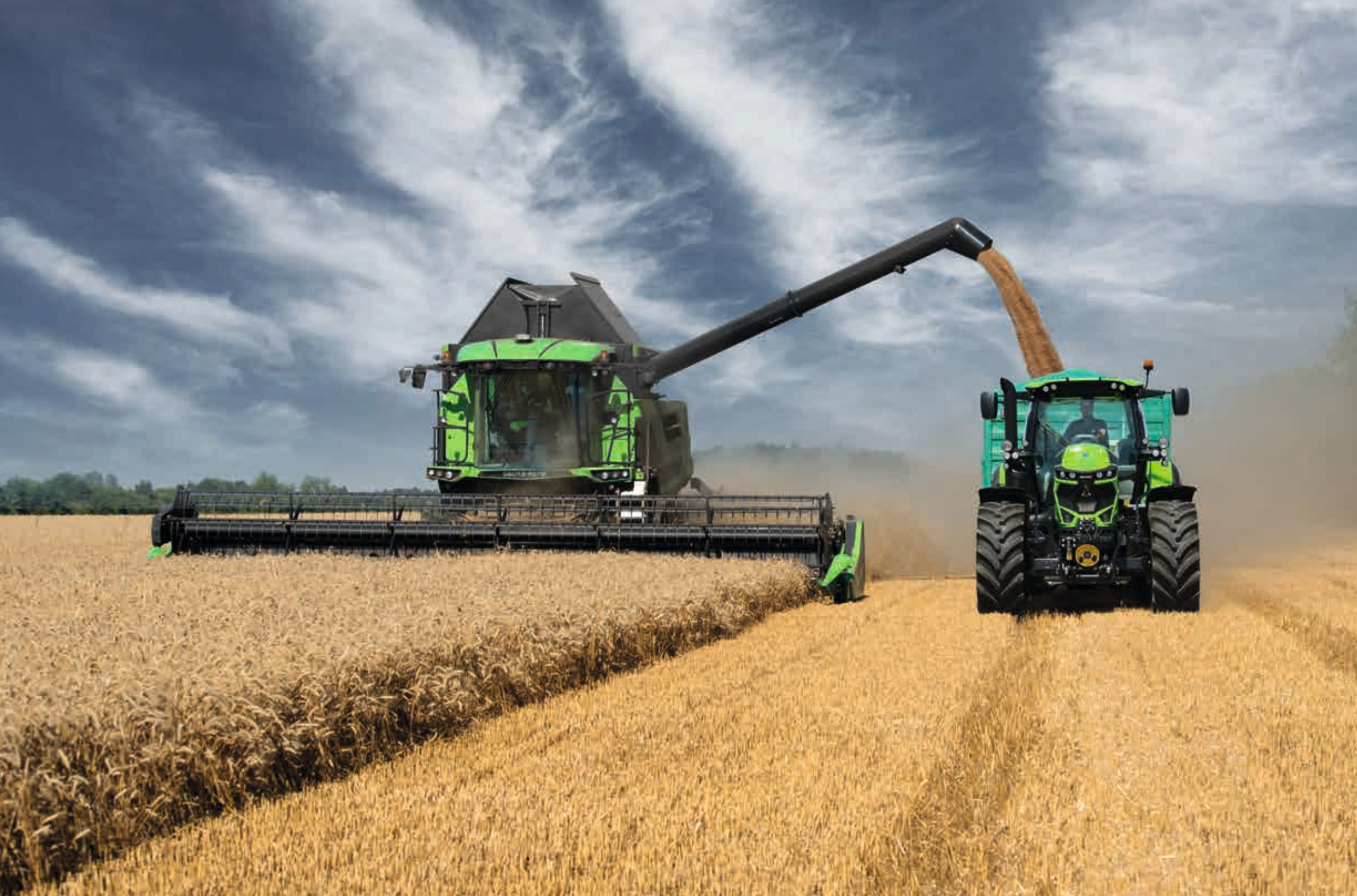
Big feeding auger. Two unloading augers in the grain tank to rapidly empty the grain tank.
