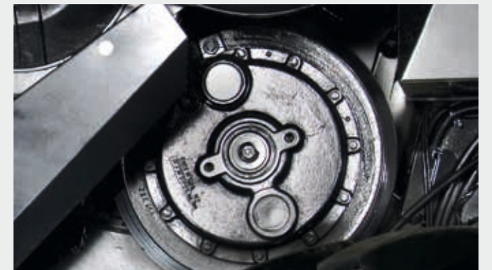
Optional threshing drum speed reducer to set the threshing drum rpm from 1250 to 625 as maximum speed and from 420 to 210 rpm as minimum speed. This kit is suggested while harvesting maize.
