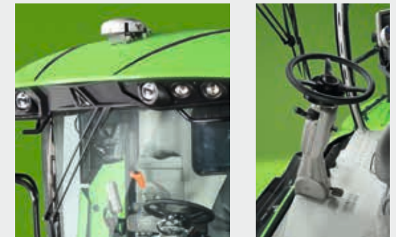
Easy installation of the precision farming systems, full integration of the electrical steering, the GPS antenna, the yield sensors and the Isobus ECU.
