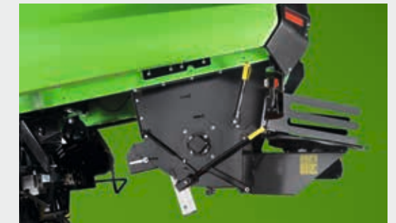
Big straw-hood discharge chute to maximize the product flow of the long straw.
