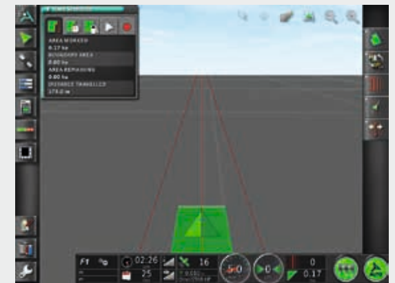
12" iMonitor integrates the software to manage Agrosky and Yield monitor.
