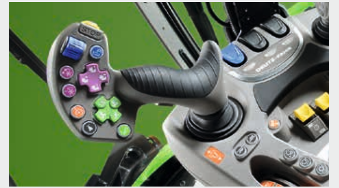
➤ The COMMANDER STICK, controls all main functions of the combine: - Header position - Reel position and speed - Unloading tube (position and discharge) - Cruise control The COMMANDER STICK also integrates the new electronic control for the transmission, effortless, more precise and ergonomic.
