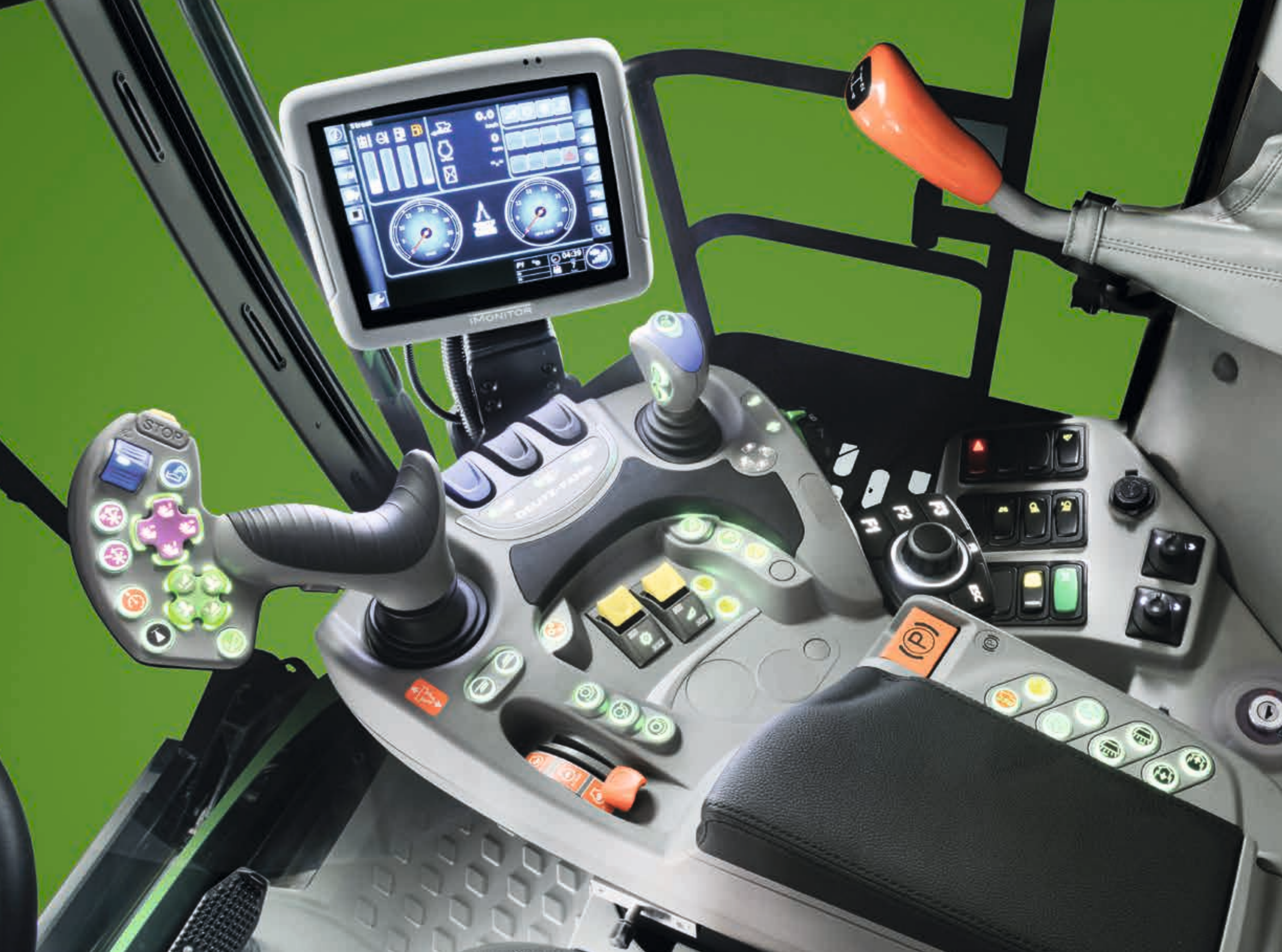
➤ The COMMANDER STICK, controls all main functions of the combine: - Header position - Reel position and speed - Unloading tube (position and discharge) - Cruise control The COMMANDER STICK also integrates the new electronic control for the transmission, effortless, more precise and ergonomic.
