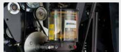
Automatic grease system with 4 kg grease pot
