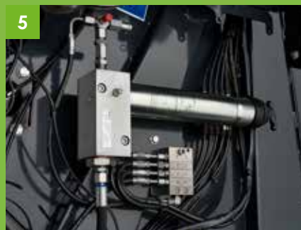
5 Standard automatic greasing system for roller bearings
