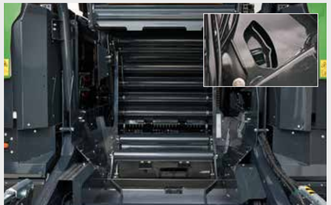
↑ The heart of the baler consists of 18 POWERTRACK rollers which generate exceptionally high densities and reliable bale rotation in all crop conditions. The rollers have built-in scrapers to push the material out and away from the bearings.
