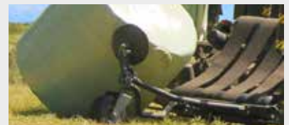
Bale turner, unloading the bale on its flat end
