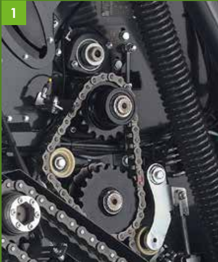
1 Second belt driven roller guarantees a secure belt drive in all crop conditions
