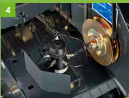
4 BEKA-MAX continuous chain oiling system
