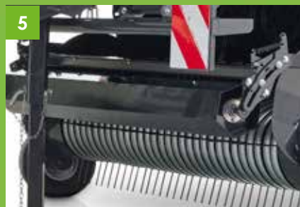
5 Heavy crop roller with wind guard (Ø 217 mm)
