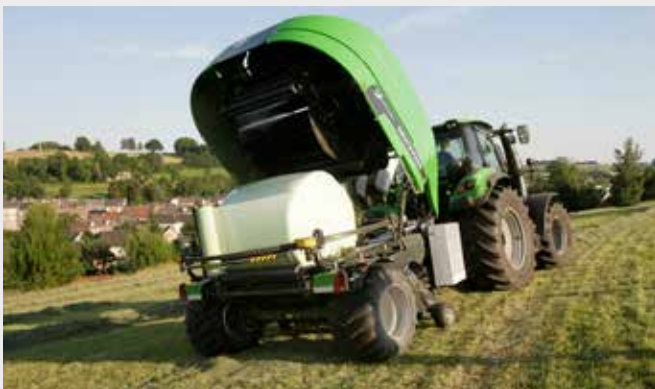
↑ The wrapping ring is unique to the COMPACMASTER+, with two integrated pre-stretchers. They rotate close around the bale with outstanding speeds (of up to 50 rpm). It only takes 18 seconds to wrap a bale with 6 layers of film.
