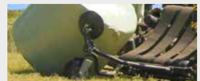
Bale turner, unloading the bale on its flat end
