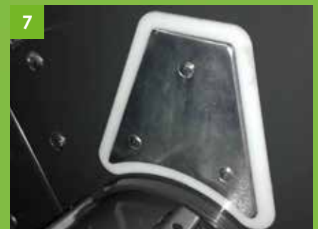
7 i-DENSE system automatically adapts the baling pressure based on moisture sensor measurements
