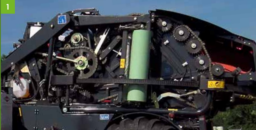
1 Robust driveline with high quality IWIS chains
