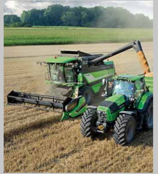
Unloading tube to discharge the grain while working in any position to tall trailer.
