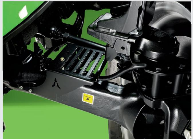
↑ Maintenance steps above the front axle for comfortable cleaning.
