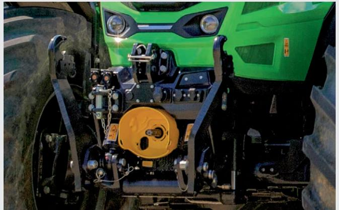
5,450 kg lifting capacity and dual speed front PTO.
