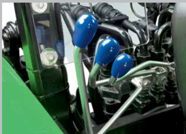
Equipped with up to 3 mechanical auxiliary valves.
