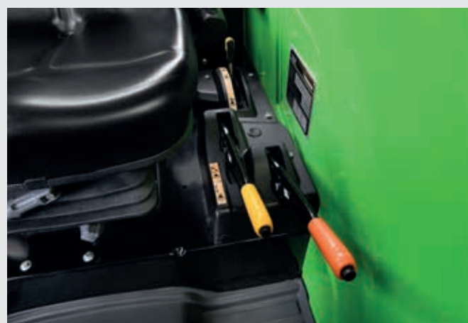
↑ Mechanical PTO speed selector and engagement.
