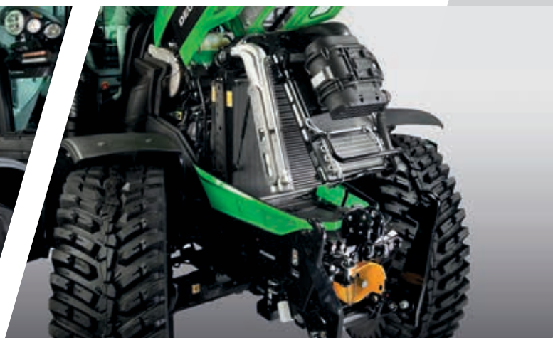
> Aluminium cooling system Performance Pro with one-hand release lever for models 6210-6230.
