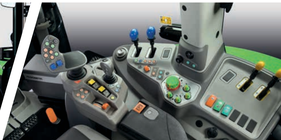
> Mixed configuration with 2 mechanical distributors and 2 electric ones.
