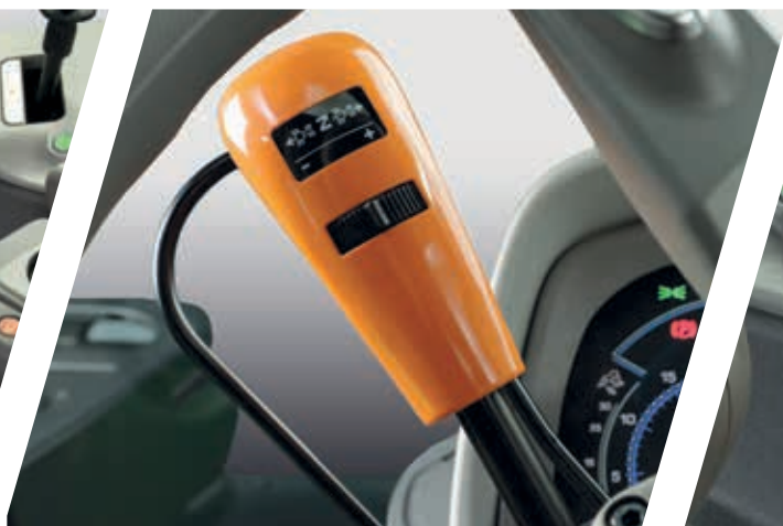
> PowerShuttle lever with SenseClutch adjustment dial.
