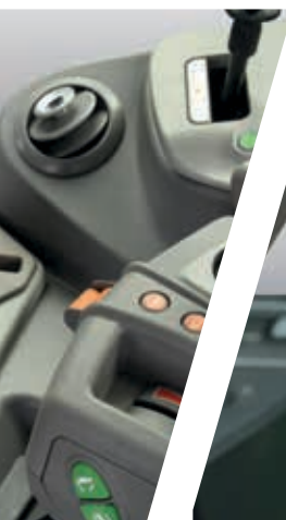
> PowerShuttle lever with SenseClutch adjustment dial.
