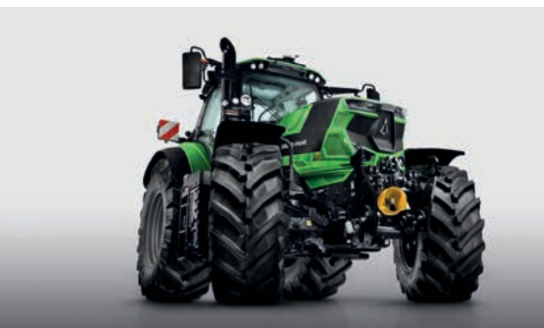
> Front suspended axle with 100% front differential lock.
