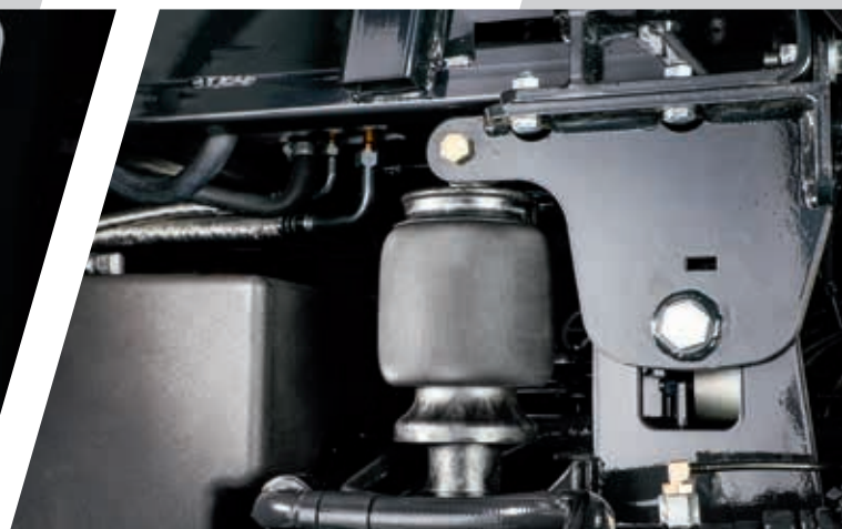
> Pneumatic cab suspension for a smoother ride.
