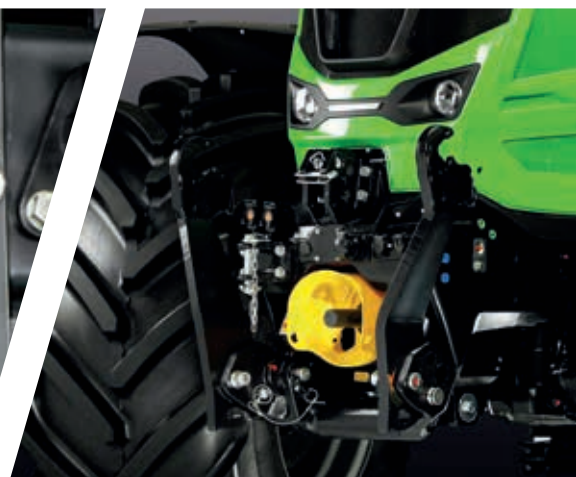
> 5450 kg lifting capacity and DualSpeed front PTO.
