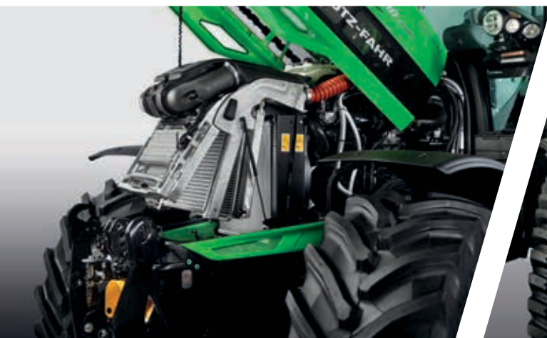
> Aluminium cooling system Performance + with one-hand release lever for models 6160-6190.
