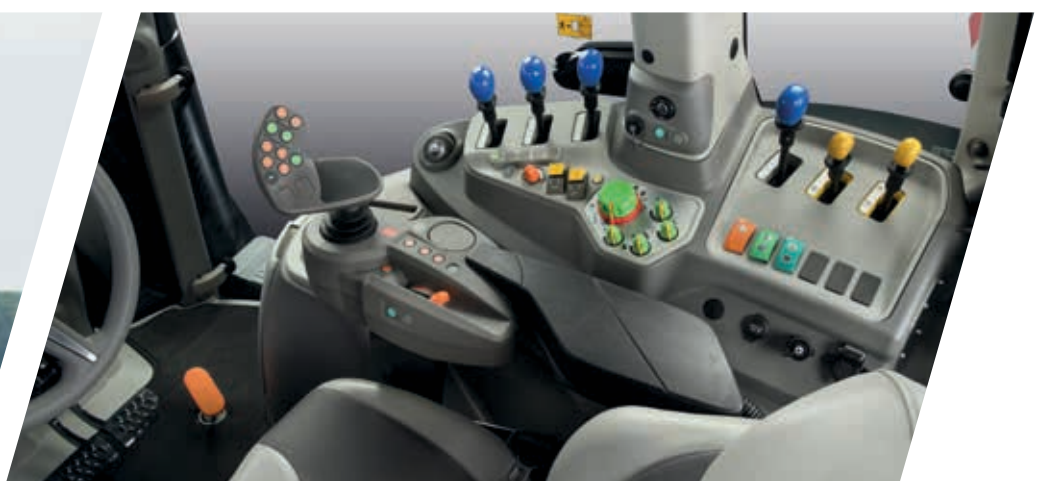
> MaxiVision cab equipment with full mechanical rear spool valves in combination with Powershift (large picture) and RCshift (picture above) transmission.
