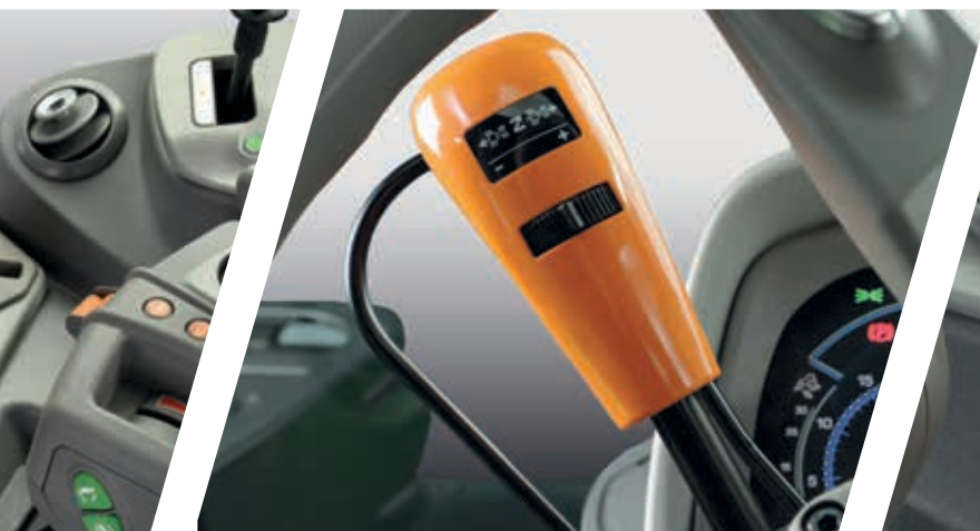
> PowerShuttle lever with SenseClutch adjustment dial.
