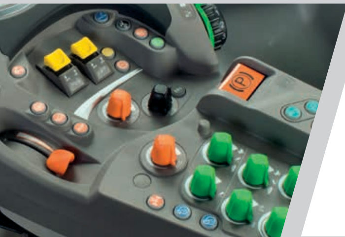
> Electronic hand throttle with two storable speed memories.
