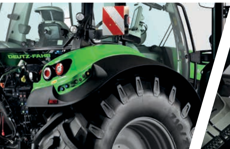
> External controls on both sides for rear lift, PTO and up to one spool valve.
