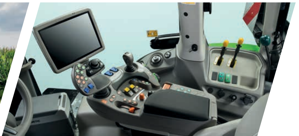
> Ergonomic MaxCom joystick with lift buttons, engine/transmission controls, headland management button and two proportional hydraulic valve control units.
