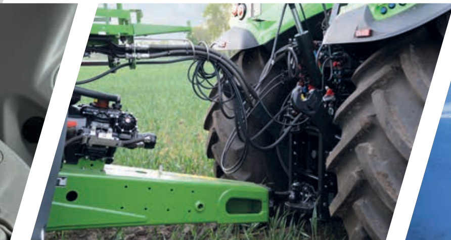
> Rear linkage with transport position so that the lower links does not collide with the drawbars when cornering (for 6190 TTV - 6230 HD TTV).
