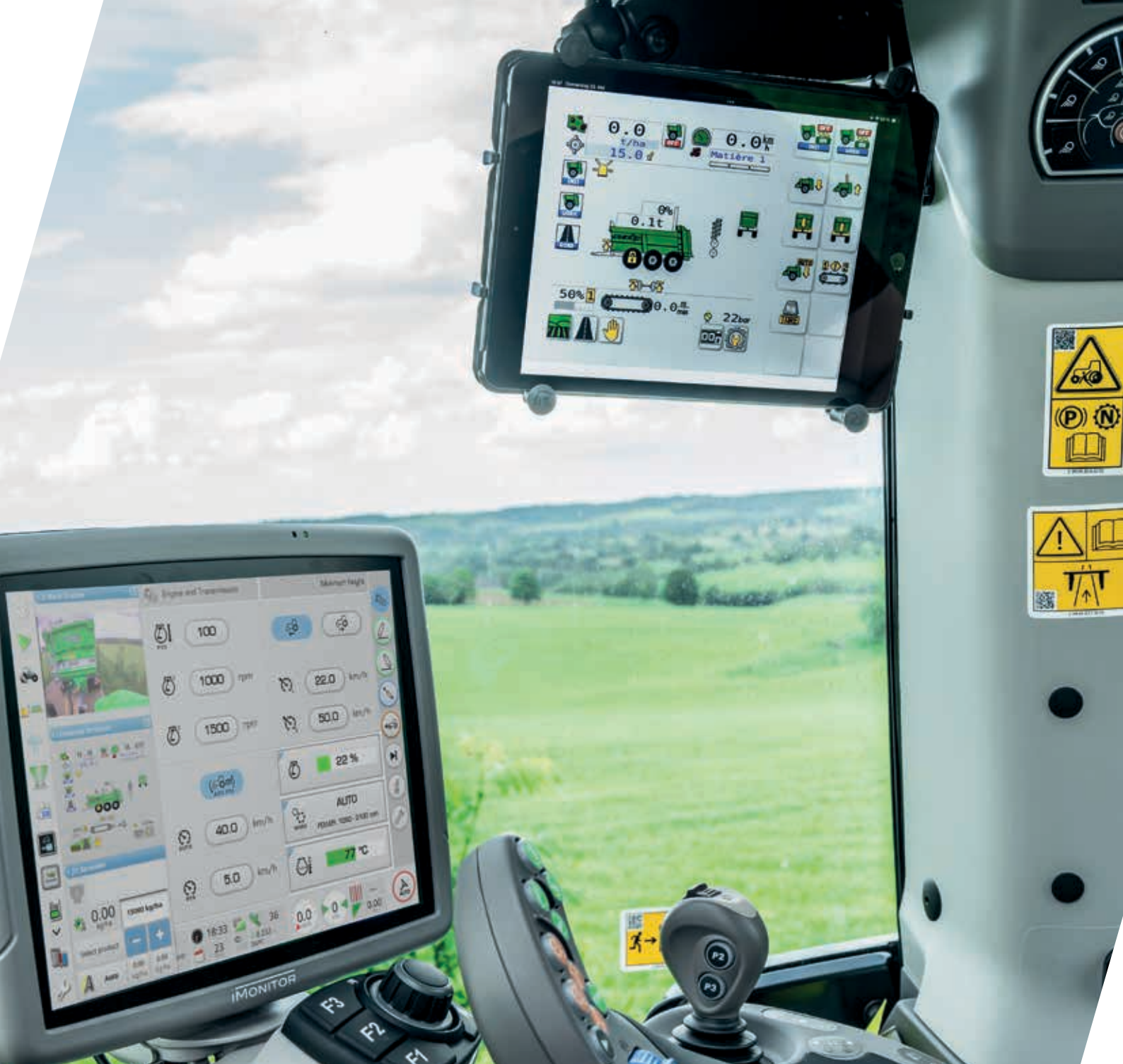
> The XTEND function allows the display of SDF Guidance or let you control an ISOBUS implement on an external device, e.g. a tablet.
