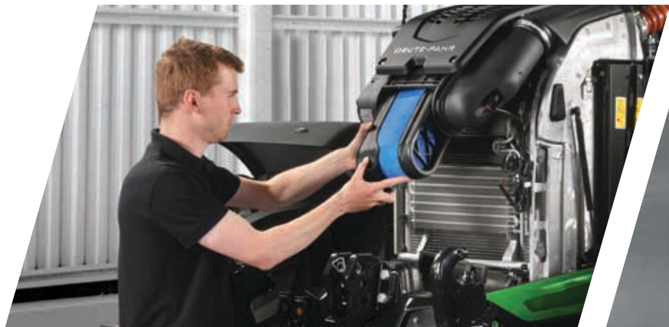
> All models are equipped with a PowerCore air filter for a long service life.
