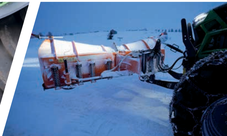
> Front lift with load relief control allows adjusting the contact pressure of the implement and reallocates weight to the front axle.
