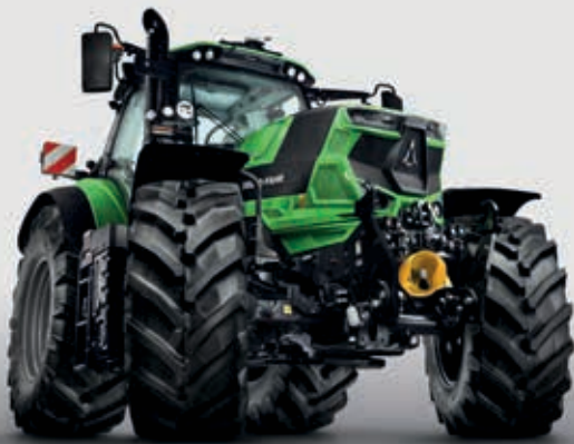
> Front suspended axle with 100% front differential lock.
