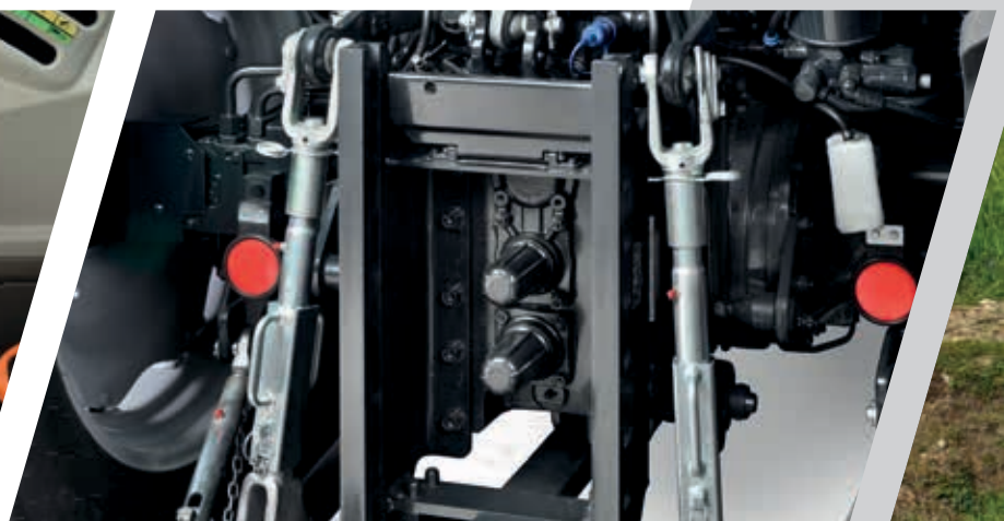
> Groundspeed PTO with independent shaft.
