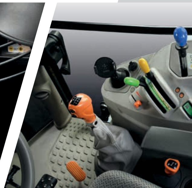
> Ergonomic and organised side control with mechanical rear lift for models 5095 - 5105 - 5105 HD.
