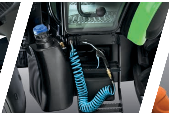
> External and in-cab air connections for air-compressor accessories.
