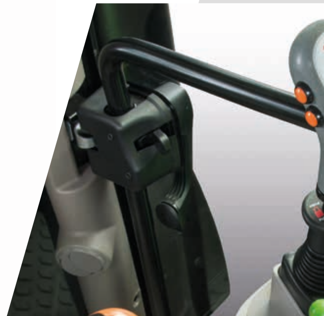
> Joystick with Powershift control for easy movement of the front loader.
