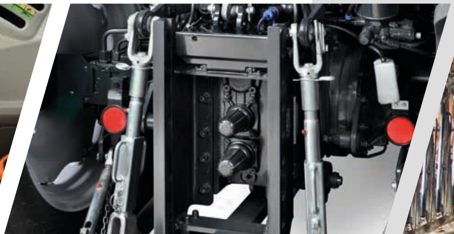
> Groundspeed PTO with independent shaft.
