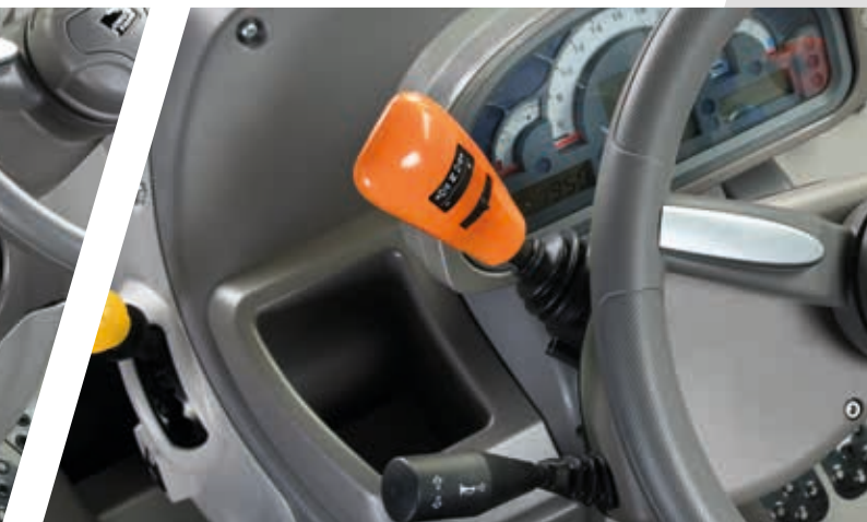
> PowerShuttle with SenseClutch 5-levels adjustment.
