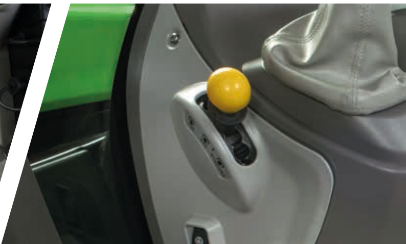
> In-cab PTO speed selector.
