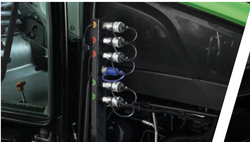
> Up to 5 mid-mounted hydraulic ways.
