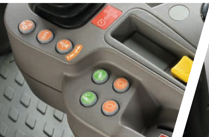
> Transport, Field, Creeper driving modes selection.
