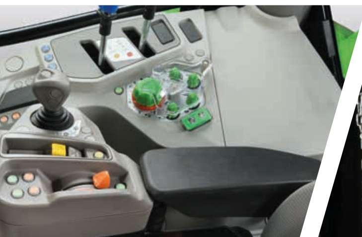
> Mechanical and electronic hydraulic controls.
