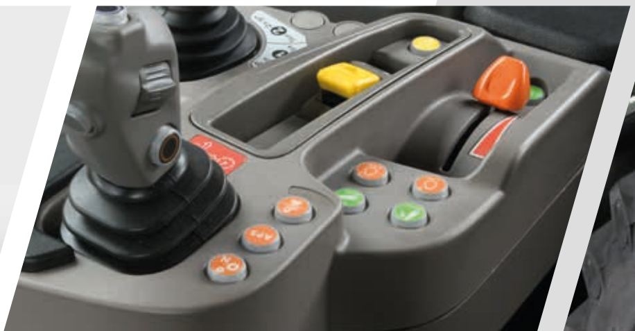
> Electronic hand throttle with 2 engine memory speeds.
