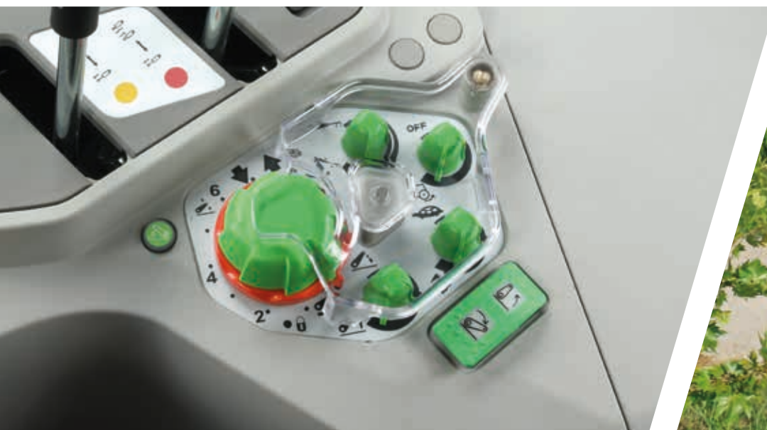
> Electronic rear lift controls.
