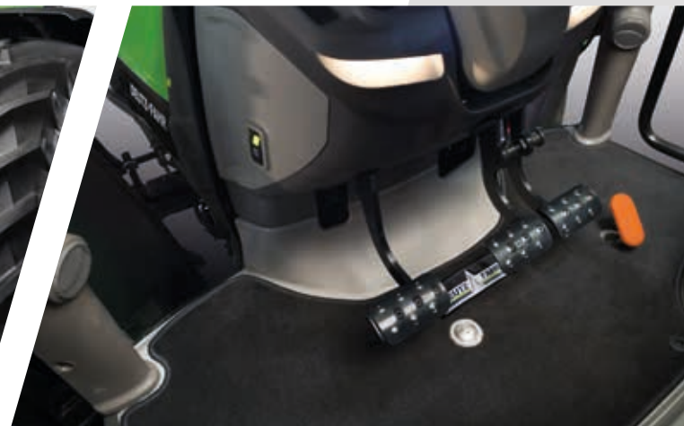
> Hydraulic Engine Brake activation.
