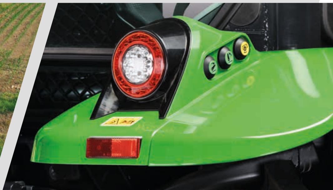
> External controls for PTO and rear lift.
