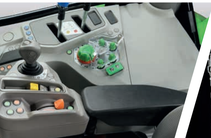
> Mechanical and electronic hydraulic controls.
