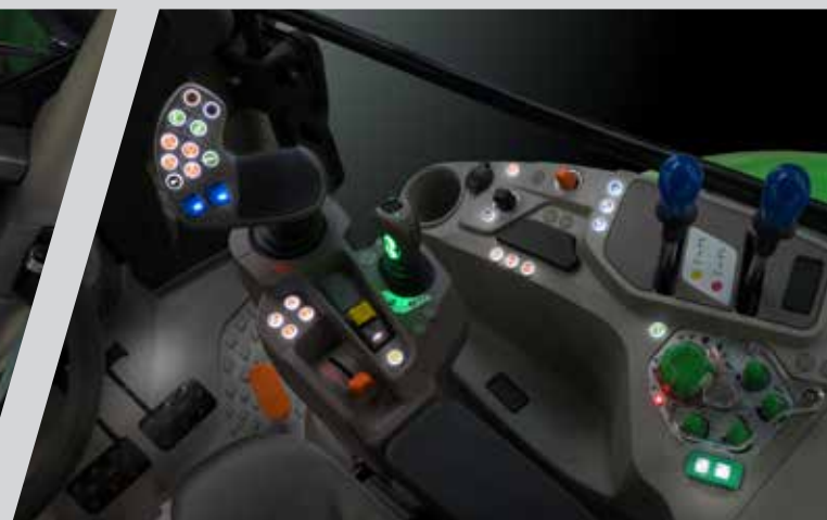
> The acclaimed MaxCom joystick equipping TTV versions is a concentrated package of high technology which lets the driver control all the main functions of the machine in complete comfort with a single hand.
