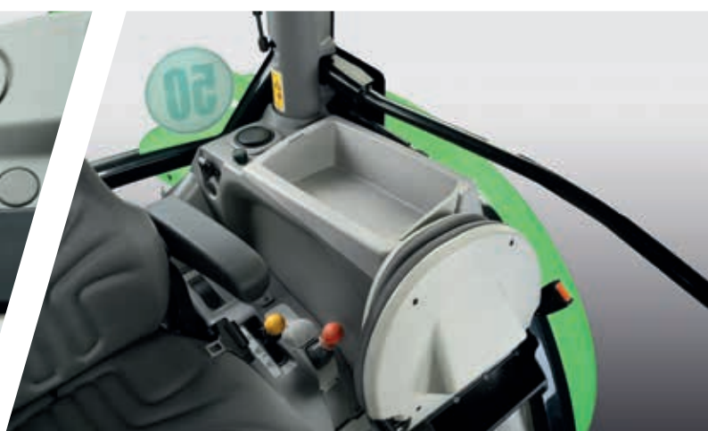
> Left console with flat storage area or portable cooling box.
