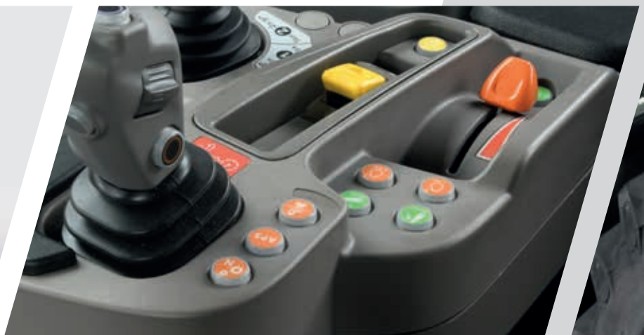
> Electronic hand throttle with 2 engine memory speeds.
