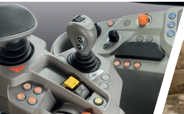
> Electronic joystick for front loader control.
