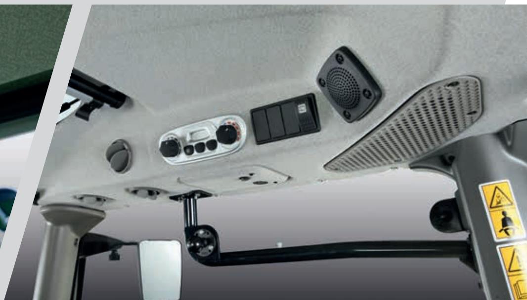
> Manual A/C and bracket for external monitor/device.
