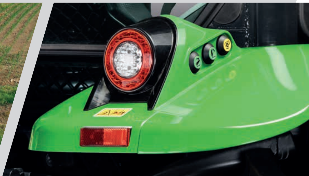
> External controls for PTO and rear lift.
