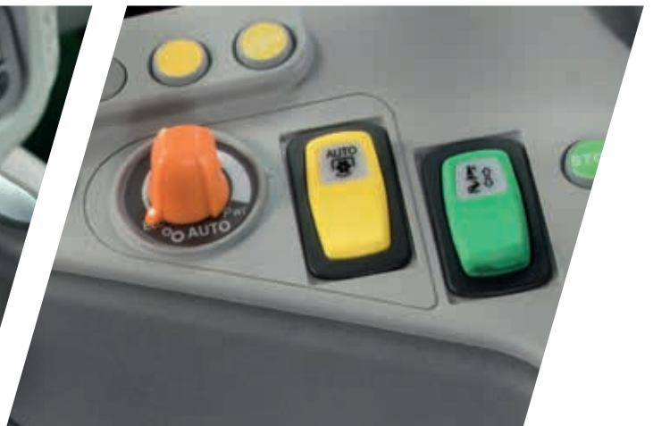
> Easy and intuitive – with the ECO/Power adjustment knob the operator can change the APS (Automatic Powershift) shifting behaviour.
