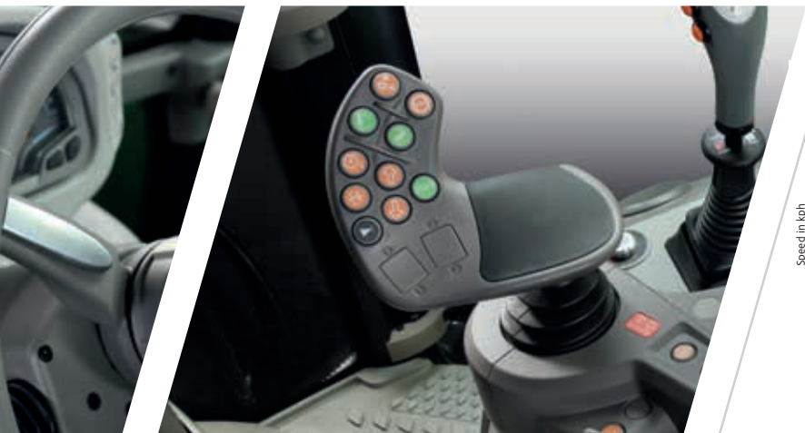
> Simple and intuitive transmission management through the practical and ergonomic MaxCom joystick.
