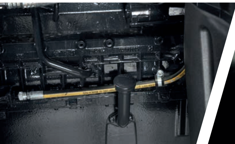
> Engine oil dipstick accessible without opening the bonnet.
