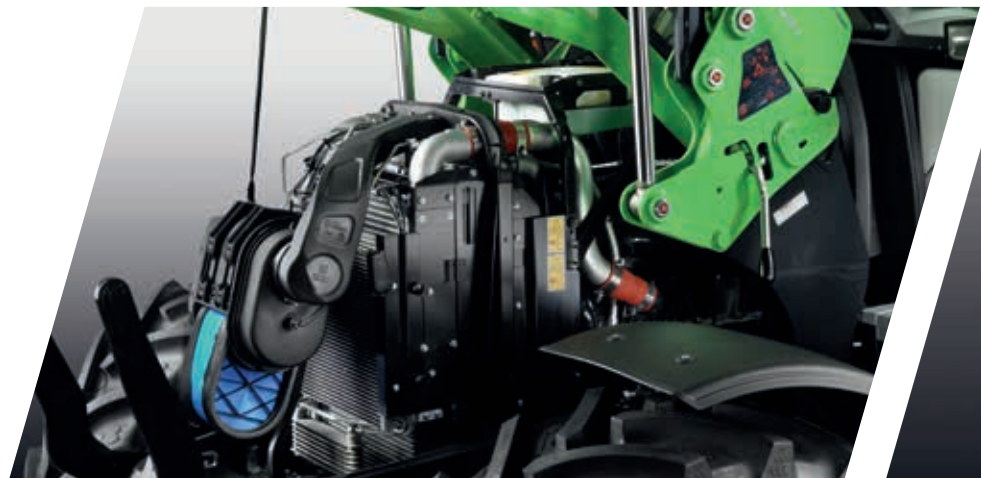
> Easy access to the PowerCore air filter and the radiator package.
