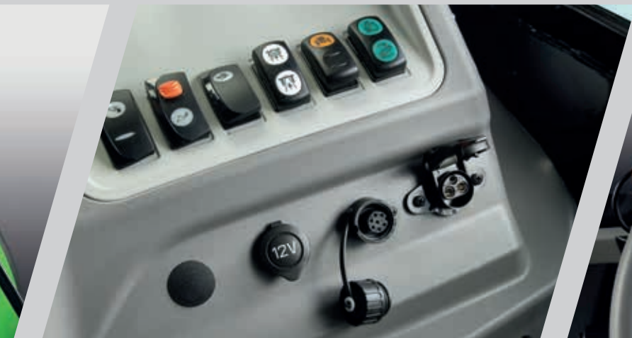
> Front loader control buttons and electrical sockets.
