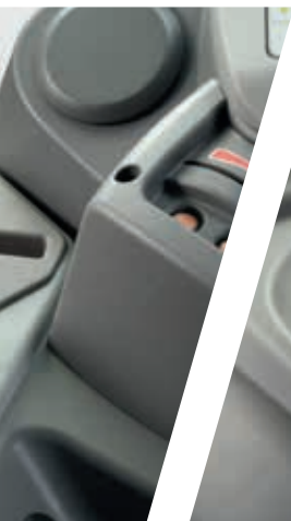
> Ergonomic PowerShuttle lever with SenseClutch adjustment dial.
