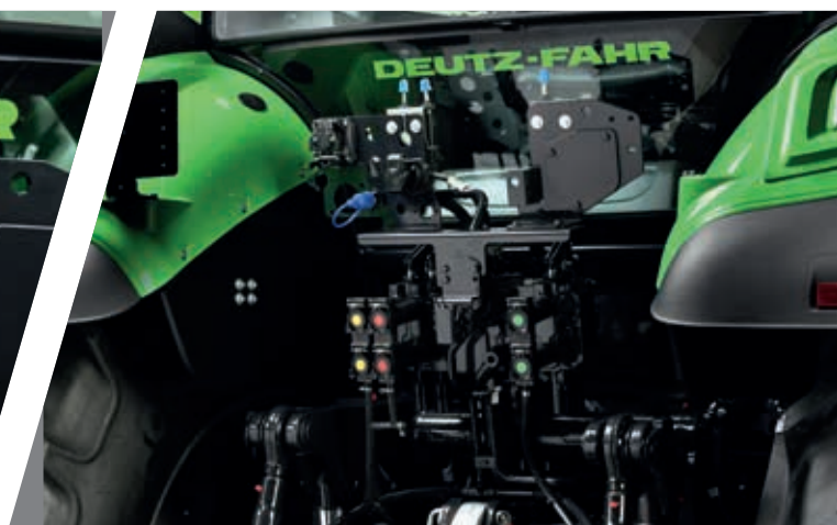
> Rear attachment area with three mechanical valves.
