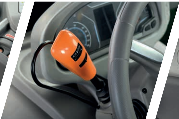
> Ergonomic PowerShuttle lever with SenseClutch adjustment dial.
