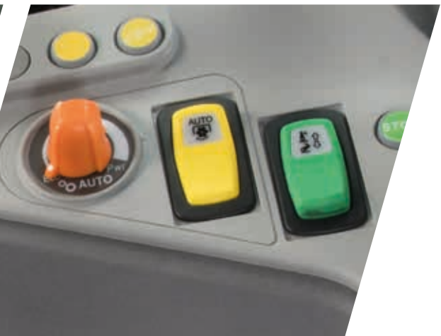
> Easy and intuitive – with the ECO/Power adjustment knob the operator can change the APS (Automatic Powershift) shifting behaviour.
