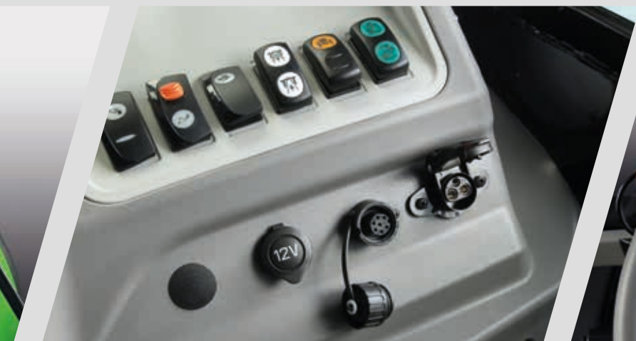
> Front loader control buttons and electrical sockets.
