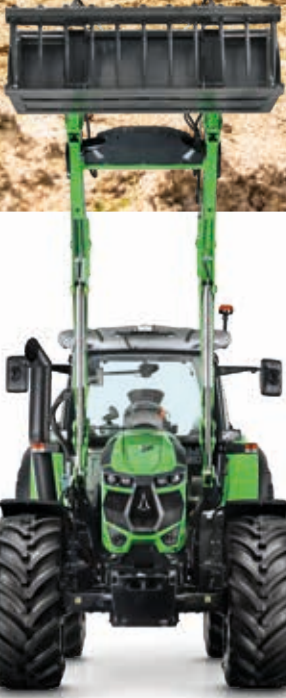
> The new ProfiLine front loaders integrate all the hydraulic lines inside the beam rail to ensure they are well protected and the driver has a clear view.
