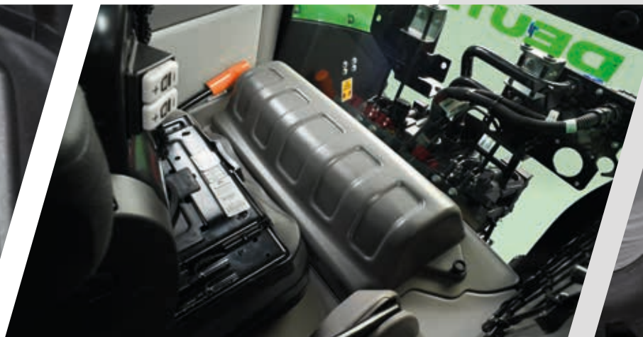
> Space behind the seat with fuse compartment and perfect view through the second rear window.
