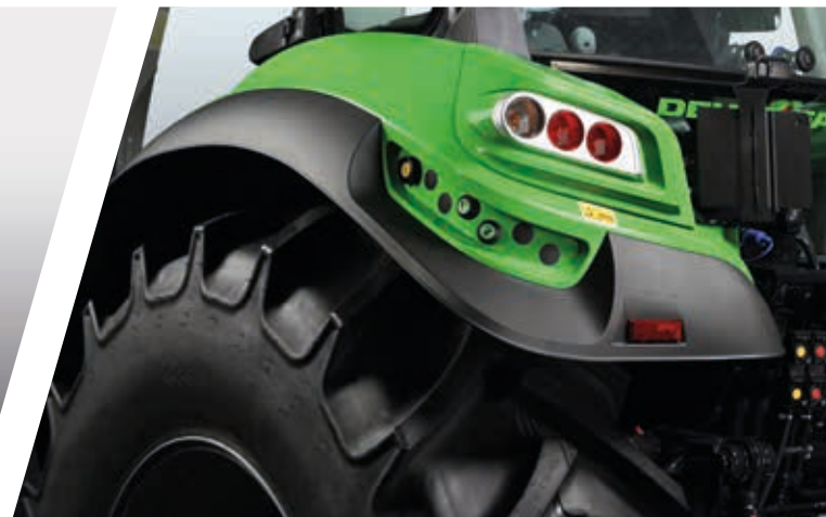
> External control elements on rear fenders for lift and PTO.
