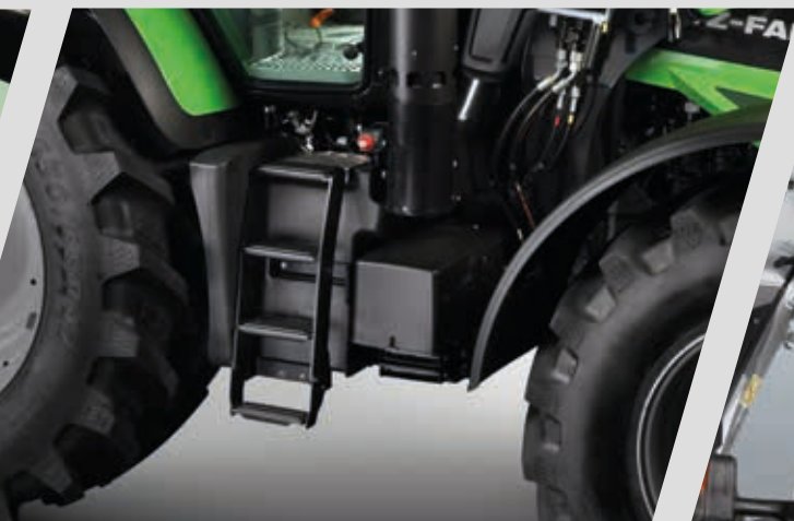
> Battery main switch and battery compartment on right tractor side.
