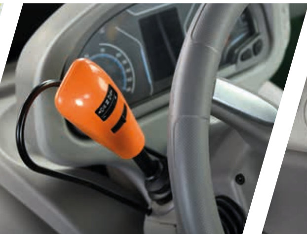
> Ergonomic PowerShuttle lever with SenseClutch adjustment dial.
