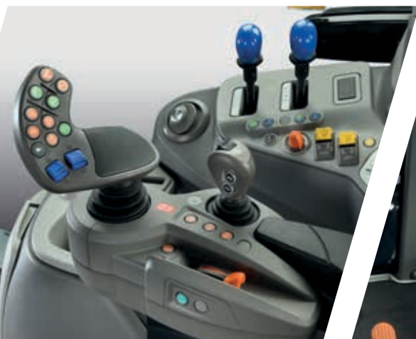
> On models with RCshift transmission the thumbwheels on the MaxCom joystick and two mechanical levers control the rear spool valves, while the cross lever might be used to control the front loader.
