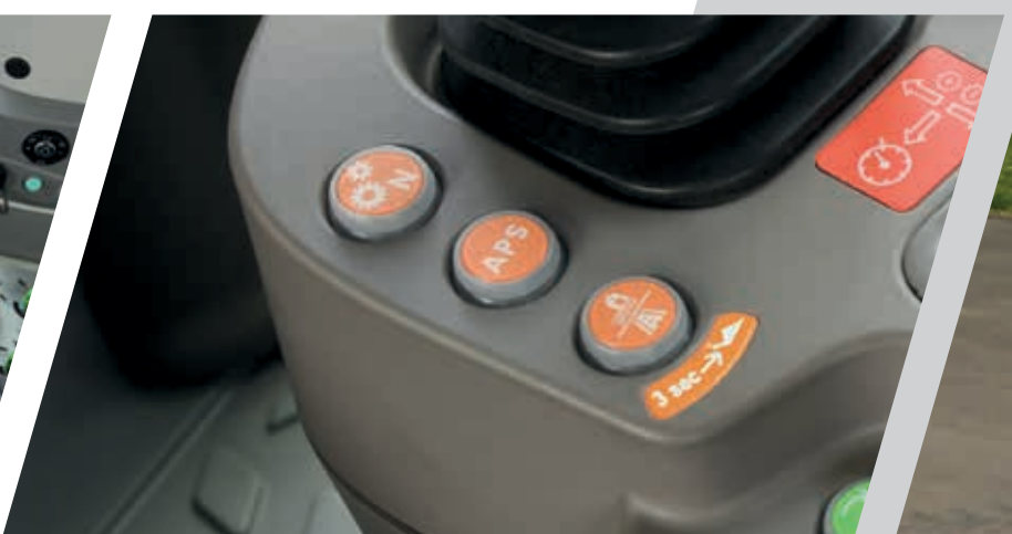
> Selection of Transport, Field and Creeper driving modes.
