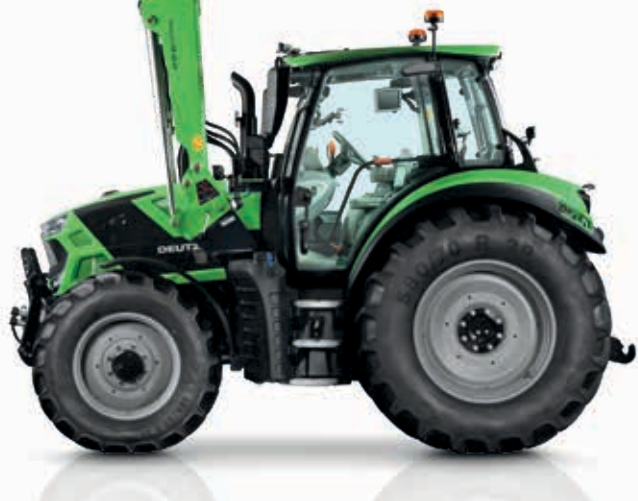
> The new ProfiLine front loaders integrate all the hydraulic lines inside the beam rail to ensure they are well protected and the driver has a clear view.
