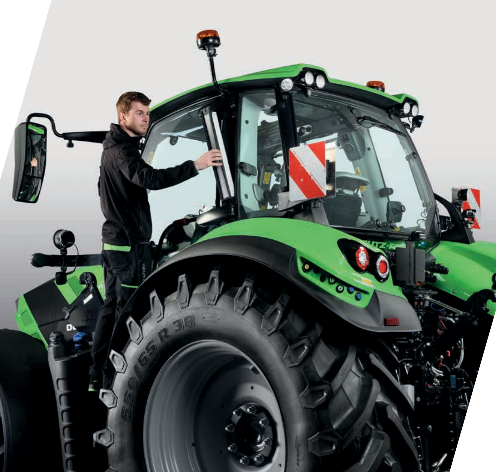
> Easy access to the large cab air filters.
