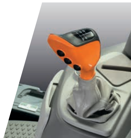
> Ergonomic gear lever with ComfortClutch, APS and Powershift buttons.
