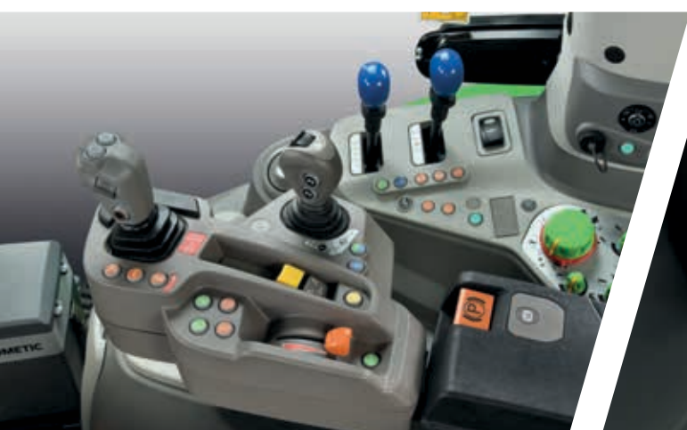
> Advanced armrest with 3 freely programmable jolly buttons and a freely programmable jolly thumbwheel.
