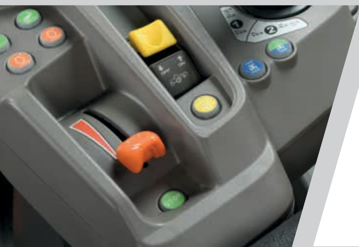
> Electronic hand throttle with two storable speed memories.
