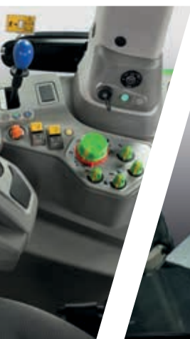
> On models with RCshift transmission the thumbwheels on the MaxCom joystick and two mechanical levers control the rear spool valves, while the cross lever might be used to control the front loader.
