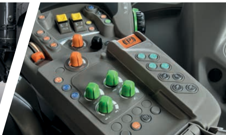
> Rear lift adjustments under armrest cover on models with MaxiVision pro cab.
