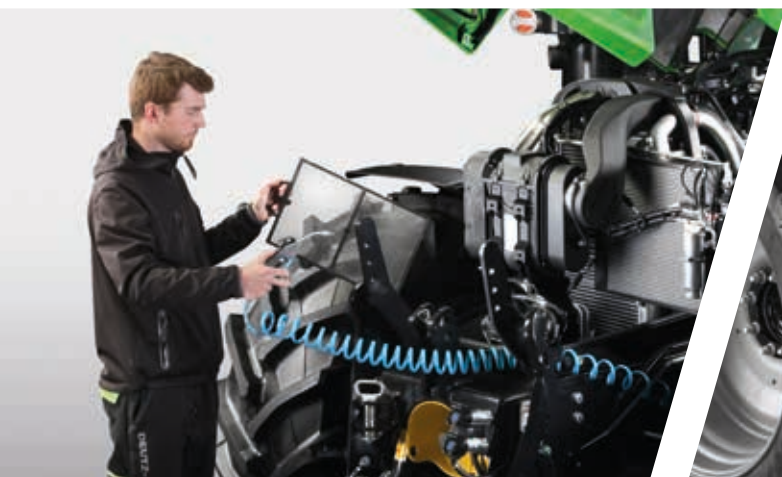
> Easy cleaning of the radiator package.
