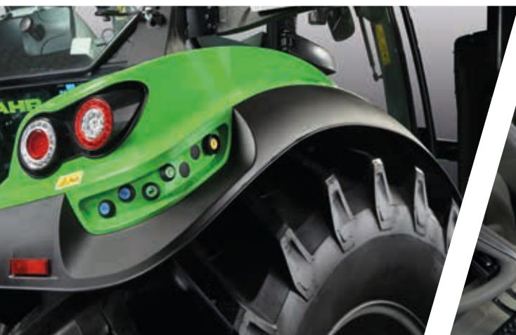
> External controls on both sides for rear lift and PTO and, depending on the model, one spool valve.
