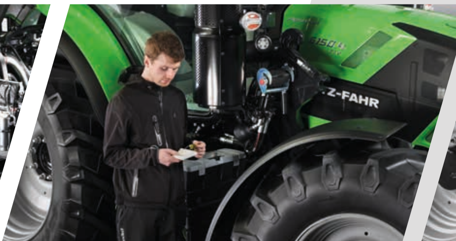
> The engine oil dipstick is accessible without opening the bonnet.
