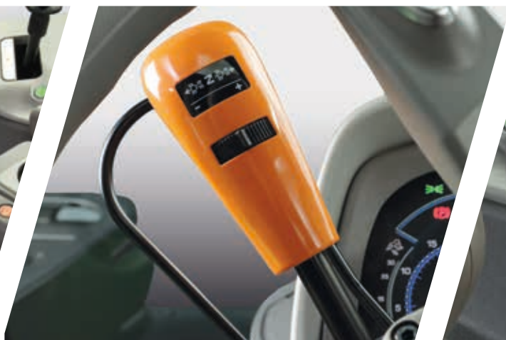
> Ergonomic PowerShuttle lever with SenseClutch adjustment dial.
