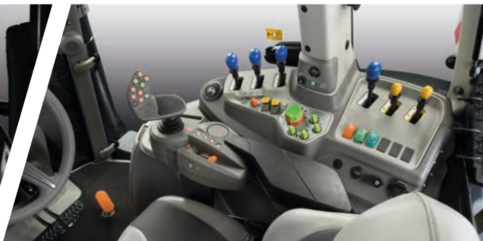
> Up to four mechanical controls with ergonomic single lever control.
