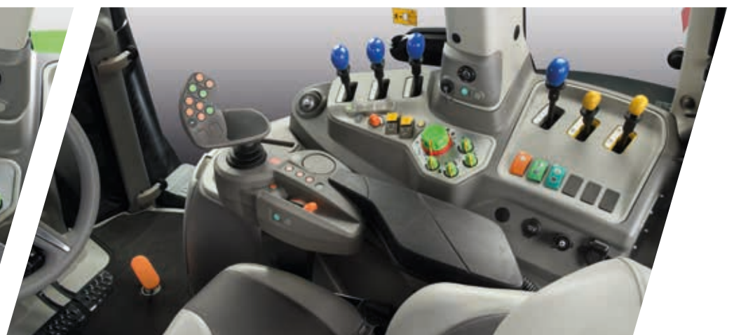
> MaxiVision cab equipment with full mechanical rear spool valves in combination with Powershift (large picture) and RCshift (picture above) transmission.
