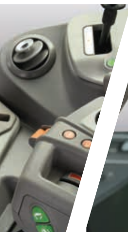
> Ergonomic PowerShuttle lever with SenseClutch adjustment dial.
