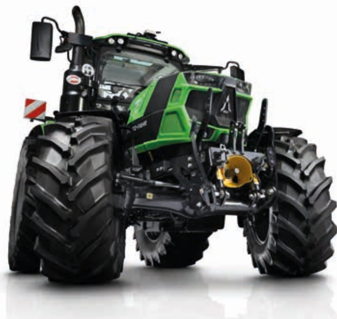
> Front suspended axle with 100% front differential lock.
