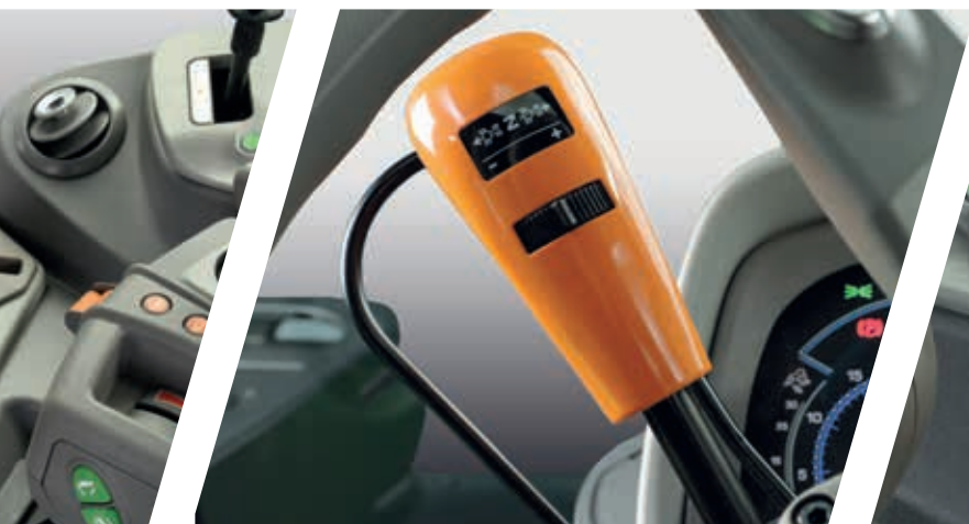
> Ergonomic PowerShuttle lever with SenseClutch adjustment dial.
