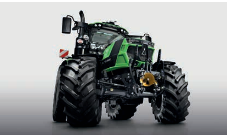
> Front suspended axle with 100% front differential lock.
