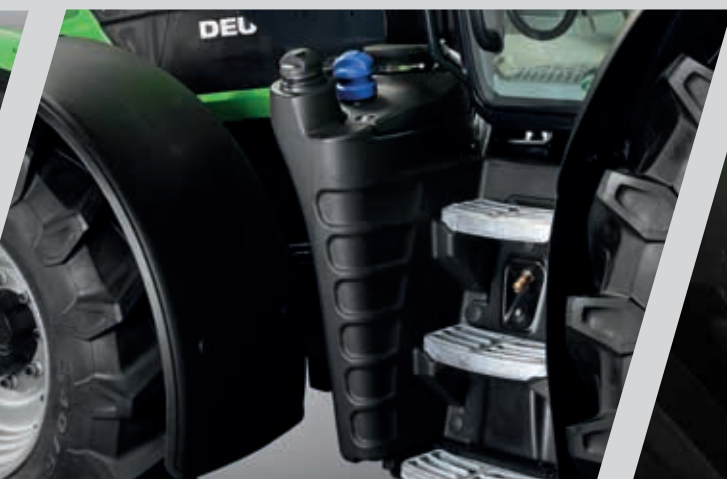
> Large fuel tank, air supply port and entrance light button between the steps for best accessibility.
