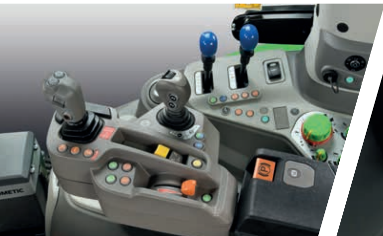
> Advanced armrest with 3 freely programmable jolly buttons and a freely programmable jolly thumbwheel.
