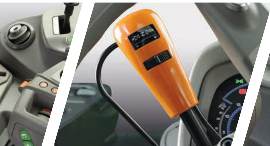
> SenseClutch ayar kadranlı ergonomik PowerShuttle kolu.
