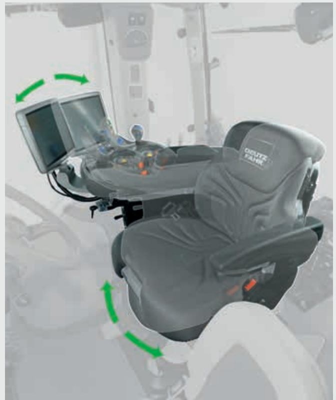
↑ Available for all TTV models: Seat with up to 23° swivel for added comfort and ease of operation.
