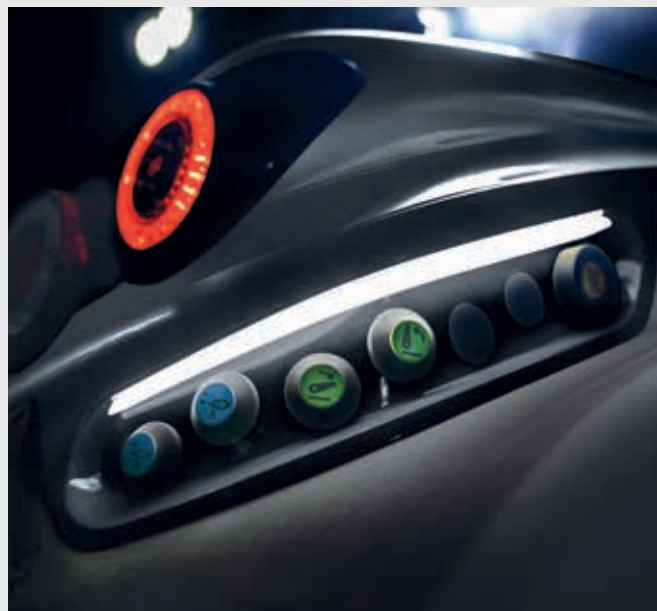
↑ LED illumination of mudguard controls.
