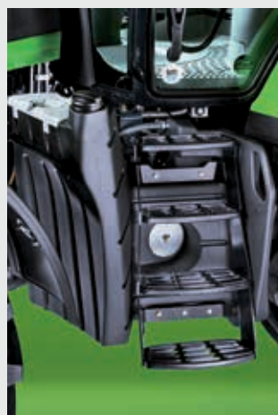
↑ Comfortable entrance steps integrated in the fuel tank.
