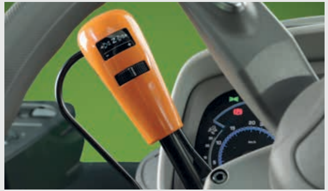
↑ PowerShuttle with SenseClutch and five adjustment levels.
