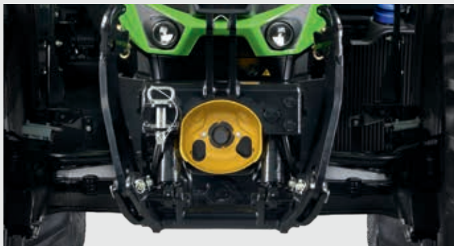
↑ Position controlled front linkage with up to 5450 Kg lifting power.
