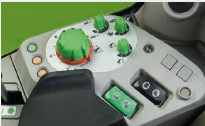
↑ Precise draft and position control thanks to electronic rear lift on cab versions.
