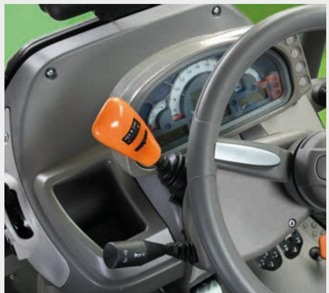
⬆ PowerShuttle with SenseClutch 5-levels adjustment.
