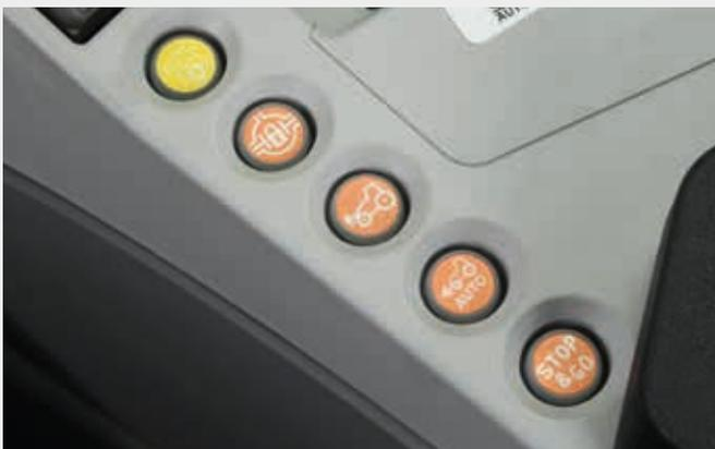
Auto 4WD function allows to engage and disengage automatically 4WD according to steering angle and speed.
