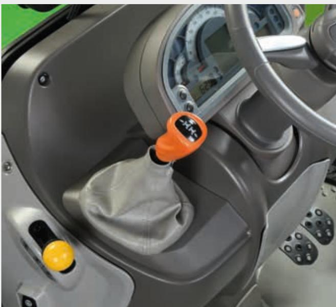
⬆ Mechanical shuttle with ergonomic lever on steering column.
