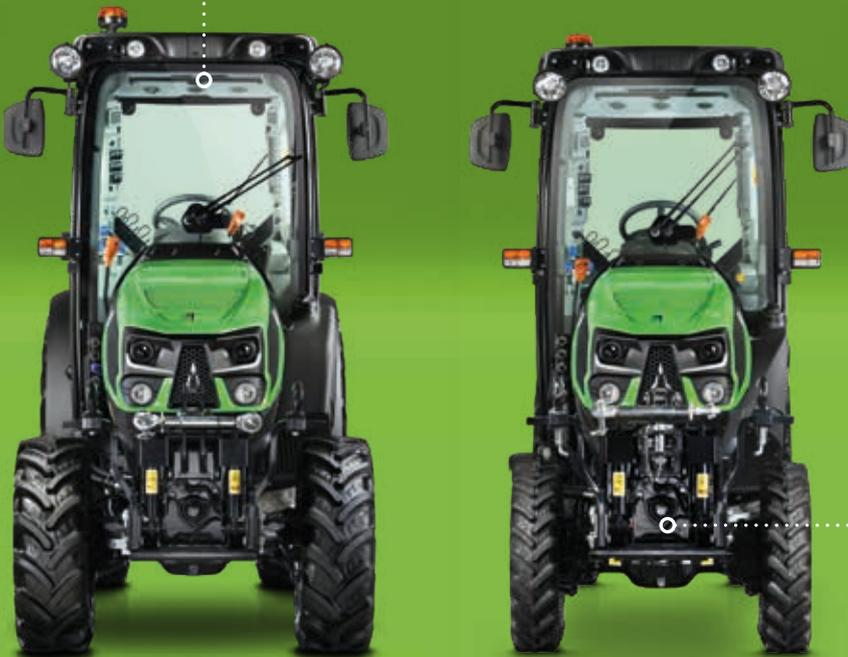
Offered with 1166 to 1671 mm width max., the new Series 5 DF/DS/DV is directed decisively towards maximum productivity and efficiency in the tightest of spaces. With new, more powerful and cost-effective 4- or 5-speed modular transmissions, 4 wheelbase lengths from 2044 to 2216 mm and powerful hydraulic systems with many variants, the new models offer greater scope for configuration, presenting themselves once again as the benchmark
