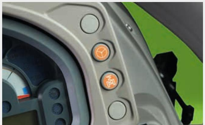
↑ SDD function halves the number of steering wheel turning required for lock-to-lock steering.
