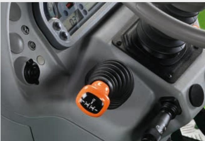
↑ Ergonomic shuttle lever under steering wheel.
