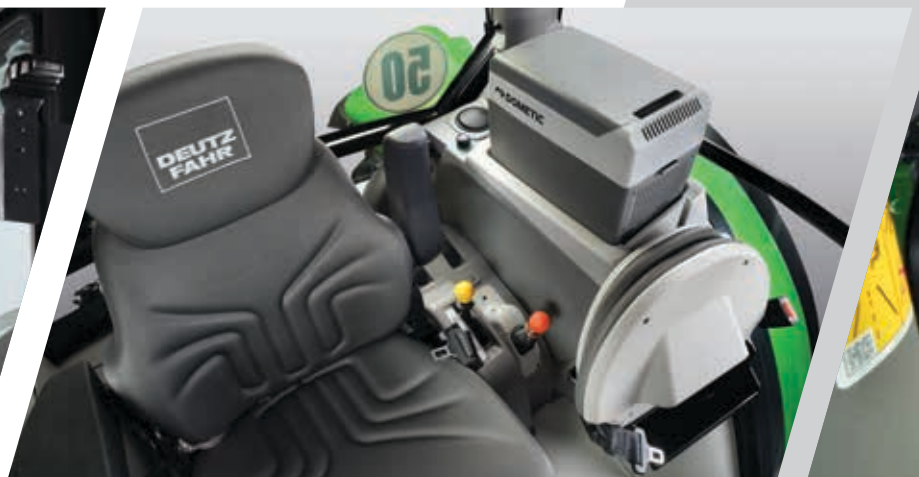
> Left console with flat storage area or portable cooling box.
