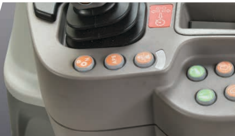
> Neutral, APS and Drive mode (Field and Road) buttons.
