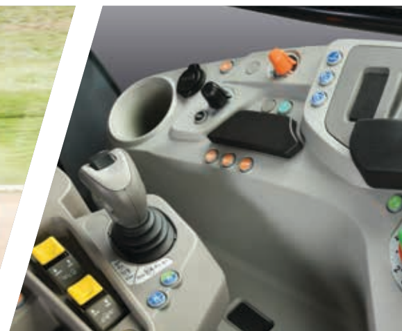
> PTO activation buttons as well as rear lift controls.
