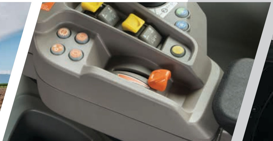
> Electronic hand throttle with 2 engine memory speeds.
