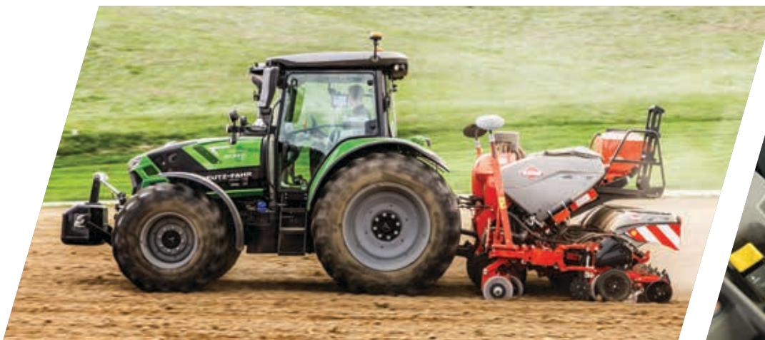
> New rear lift available for RVshift and TTV models, offering a maximum lifting capacity of 7100 kg.
