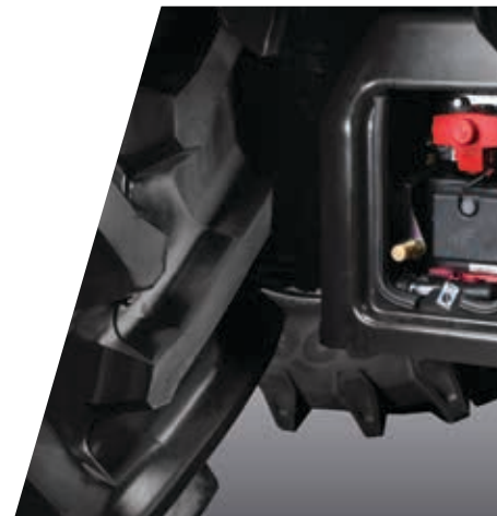
> Convenient battery port on right side.
