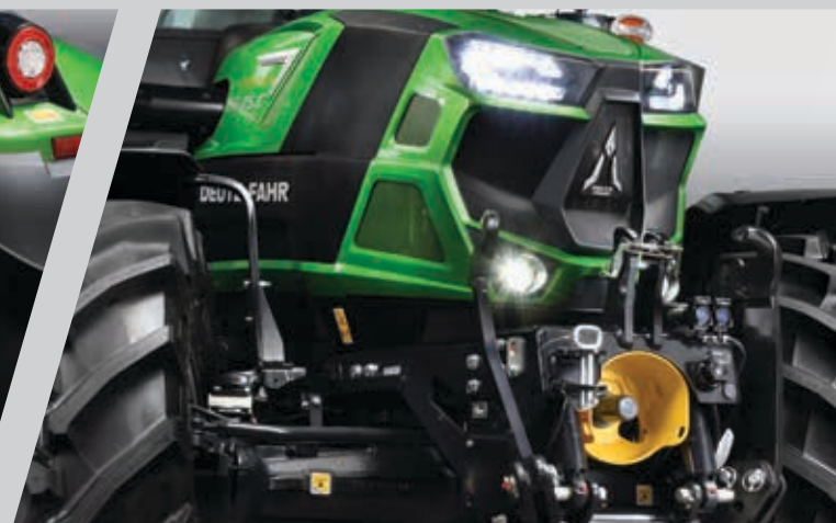
> Optional 2x front outlets in combination with front lift.
