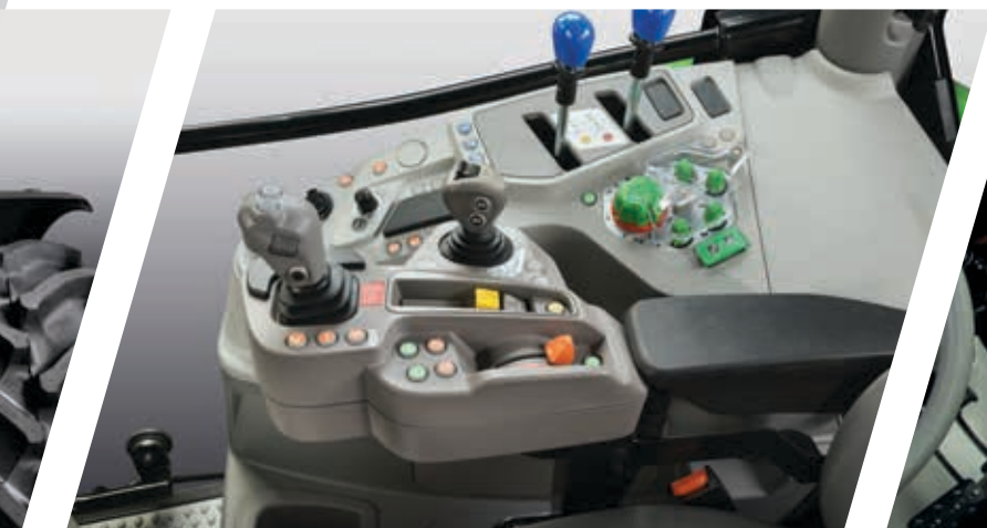
> Mixed hydraulic configuration with 2 mechanical and 2 electronic valves matched with the RVshift transmission.
