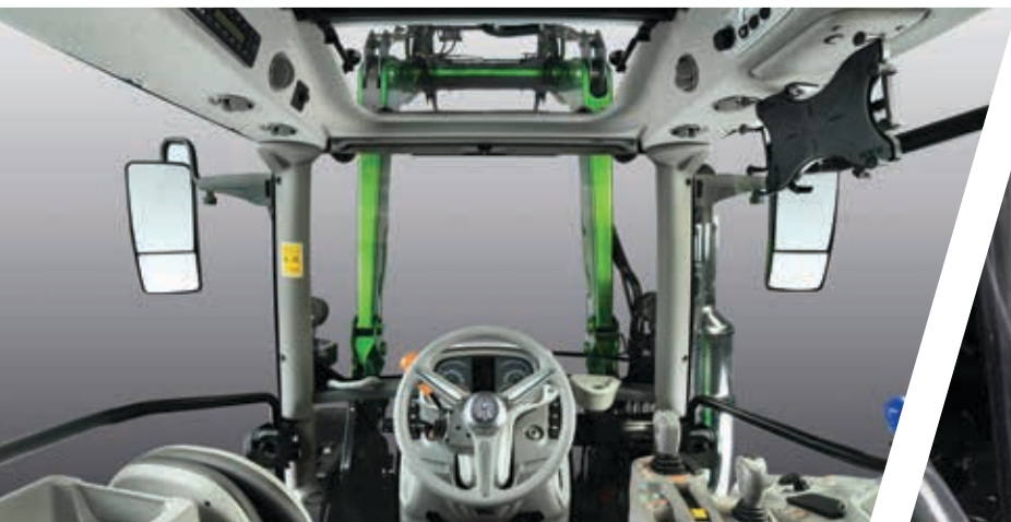
> Roof hatch and adjustable steering column.
