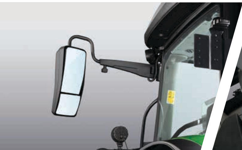
> Optional XLarge vision mirrors with electric adjustment and heating function
