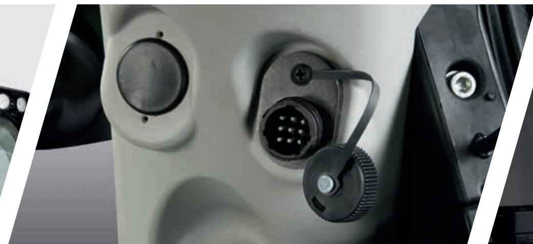
> In-cab ISOBUS plug for additional monitors.
