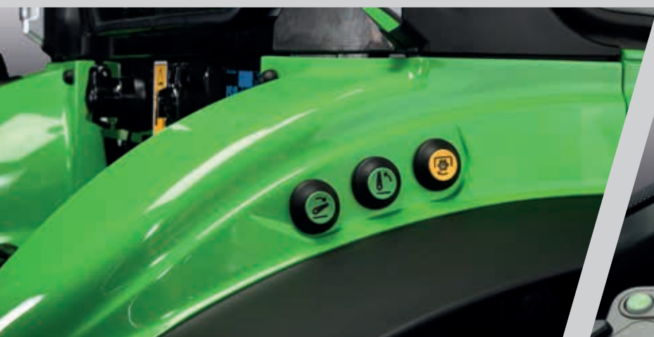
> External PTO and rear lift buttons on left and right fenders.
