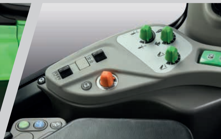
> The driver can select within a range from "ECO" engine management mode to "Power", for maximum power.
