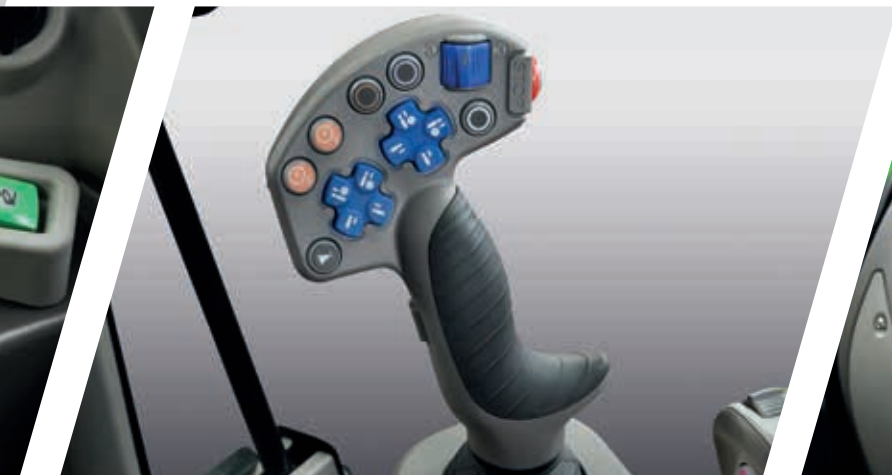
> MaxCom Joystick to allow easy management of driving speed.
