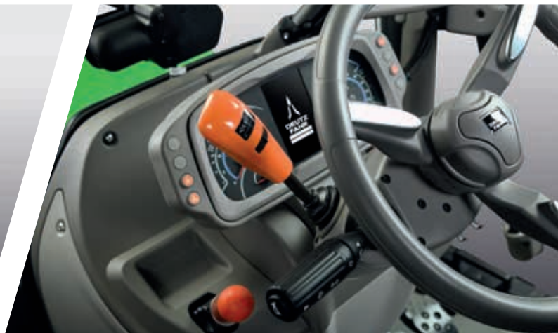
> PowerShuttle with SenseClutch (5 adjustable levels).
