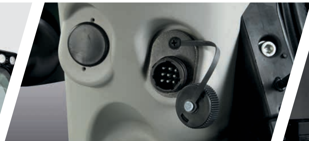
> In-cab ISOBUS plug for additional monitors.
