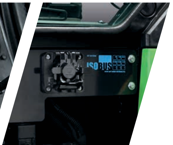
> ISOBUS: you can plug any type of implement and benefit from various ISOBUS features.
