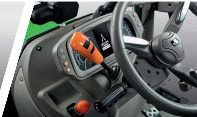
> PowerShuttle with SenseClutch (5 adjustable levels).
