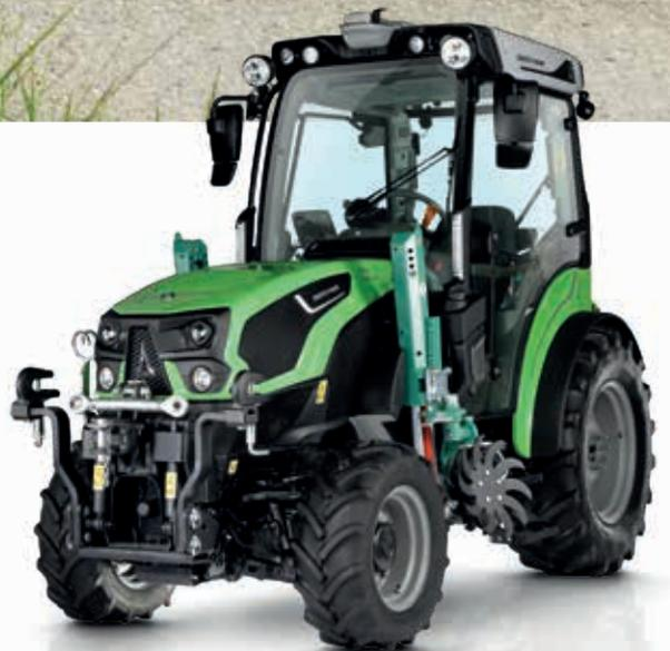
> Several sizes of PneuTrac tyres are optionally available allowing less soil compaction and higher side stability than conventional tyres.
