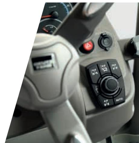
> Steering modes easily selectable thanks to the specific control on right side of steering wheels.
