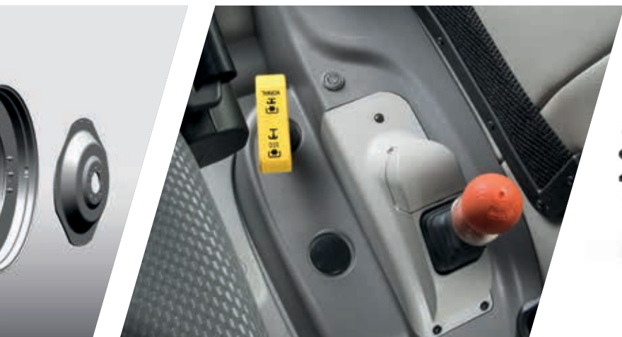
> HPB (Hydraulic Parking Brake).
