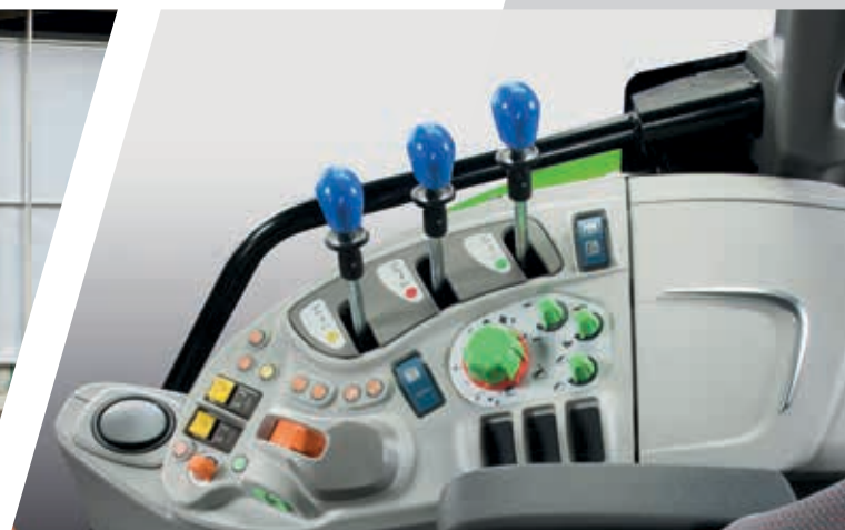
> Ergonomic layout of rear lift controls and hydraulics levers.
