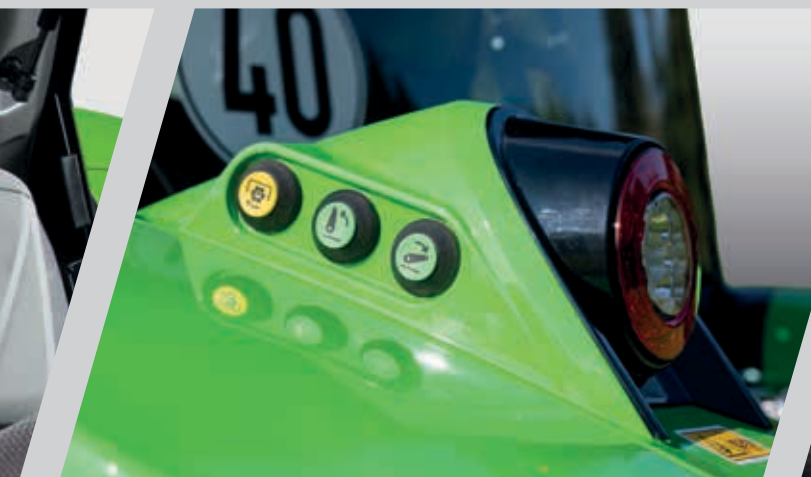
> External controls for rear lift and PTO.
