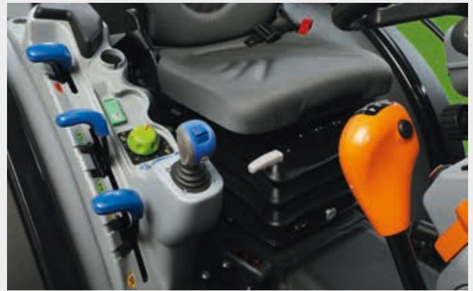
Hydraulic and rear linkage operation. Neatly arranged to the right of the seat.
