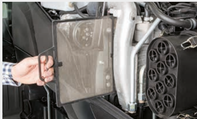
↑ The large redesigned cooling package, the improved air flow and the PowerCore air filter all support engine efficiency.
