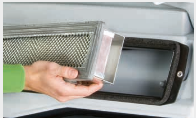
↑ Cab air filter to combat dust and chemicals. Clean air in the cab at all times.
