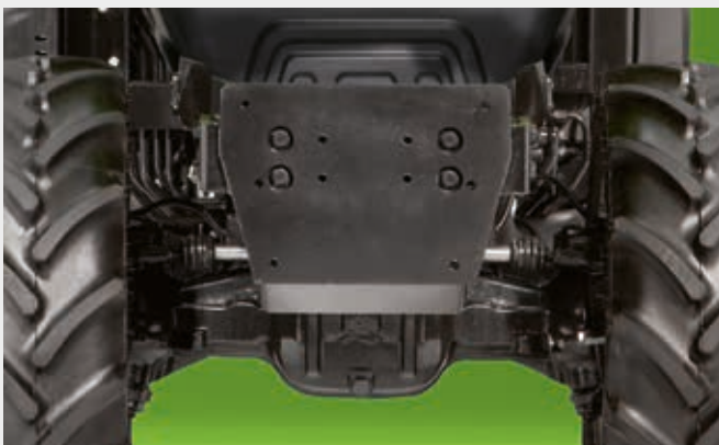
↑ Front mounting plate for quick, sturdy attachment of special equipment
