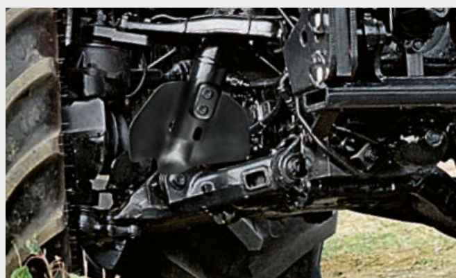
↑ Independent suspension of the front wheels with double wishbone design.
