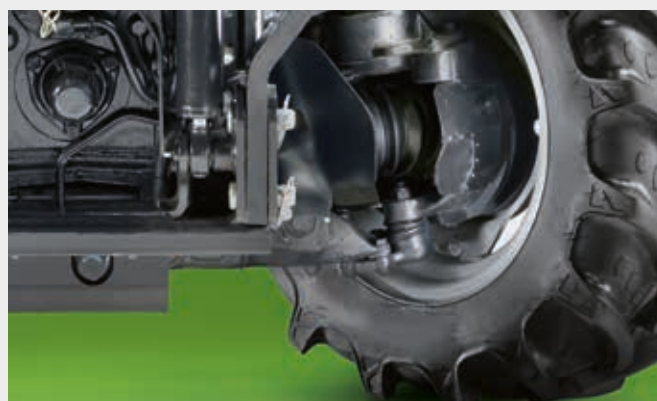
↑ 4-wheel brake system. Safety in all situations.
