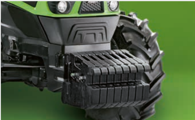
↑ A variety of front weights for working with heavy rear-mounted implements.
