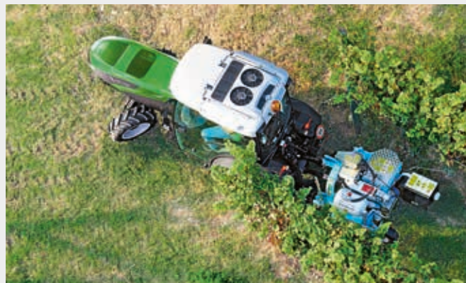
↑ Better turning radius due to slimmer geometry of the front axle frame.
