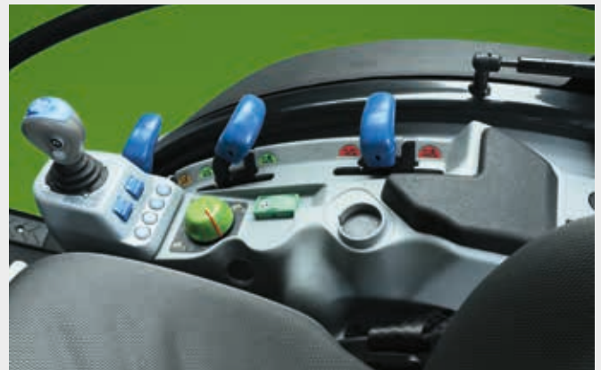
Operating lever for electronic additional control units, ergonomically positioned.
