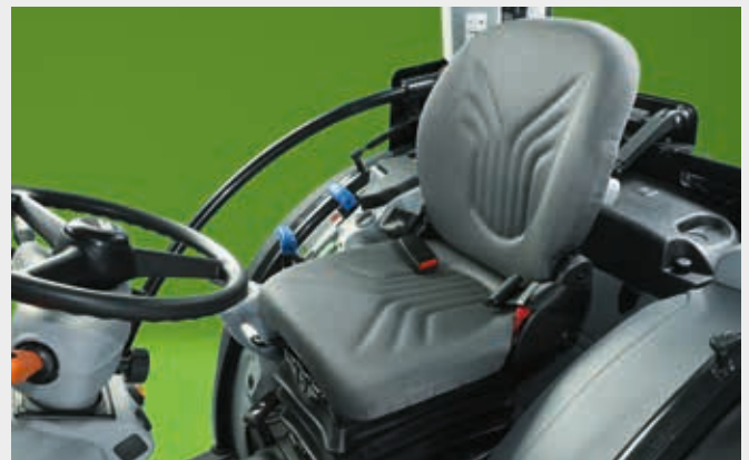
Seat variants with pneumatic or mechanical suspension and a variety of adjustment options are available.
