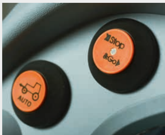
↑ Stop&Go. Convenient starting and stopping without engaging the clutch.
