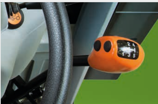
⬆ Powershift. Shifting without using the clutch, at the push of a button.
