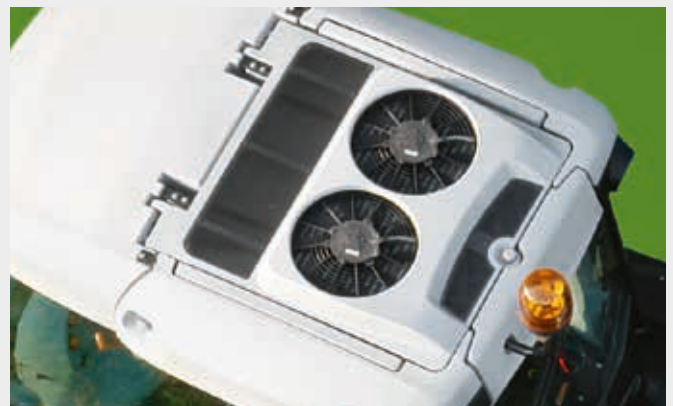
↑ Powerful air-conditioning system to guarantee a consistently good working climate in the cab.
