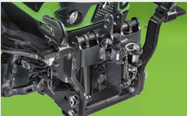
↑ Front hydraulics and front PTO for efficient equipment combinations.
