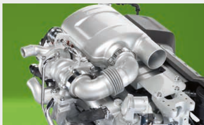
↑ Exclusive DOC system. Meets all emissions standards in one compact system without AdBlue.
