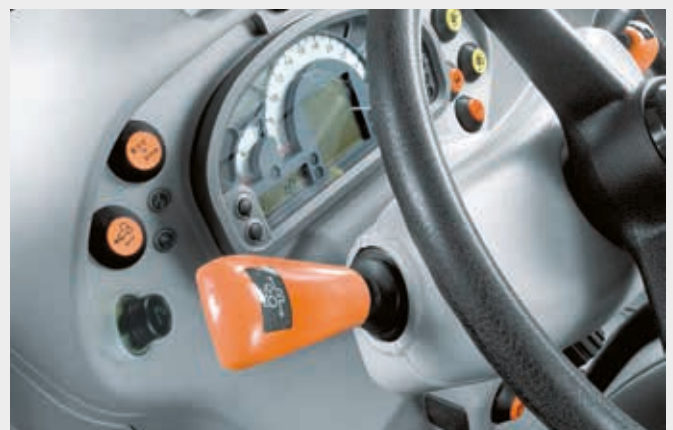
⬆ Powershuttle. Change the direction of driving in one easy step.
