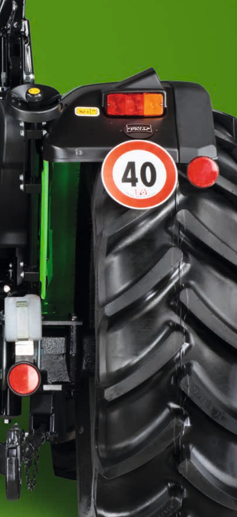
↑ The rear power lift: up to 4,525 kg lifting capacity, extremely precise control. Four rear PTO speeds as standard.
