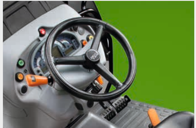
The innovative SSD rapid steering system halves the number of steering wheel turns to the full steering angle.
