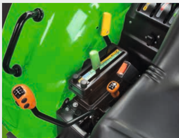
⬆ The mechanical powershift transmission with mechanical reverse shuttle is one of two transmission options.
