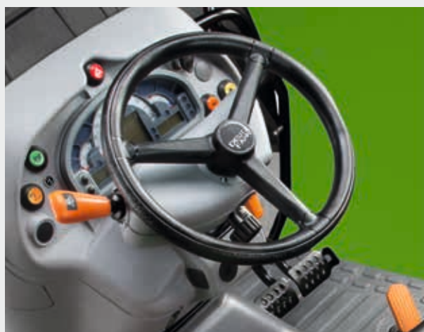
⬆ Electro-hydraulic Powershuttle system: change direction of travel without operating the clutch.
