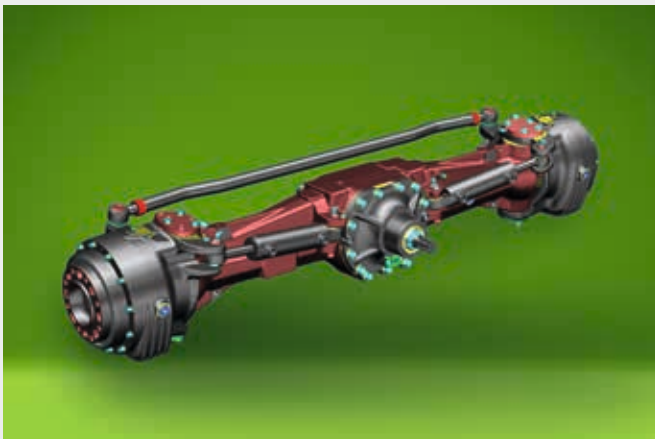
Front axle: 50-degree steering angle, electro-hydraulic all-wheel drive and differential lock activation.
