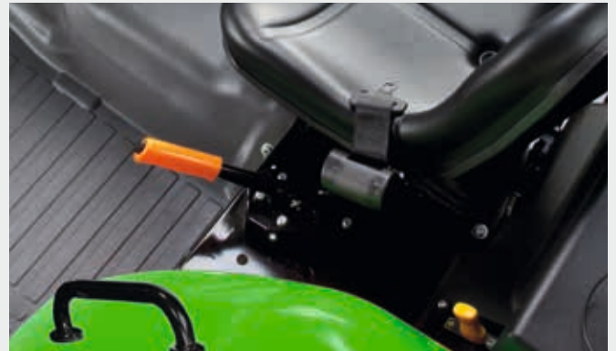
↑ To the left of the driver: parking brake and PTO controls.
