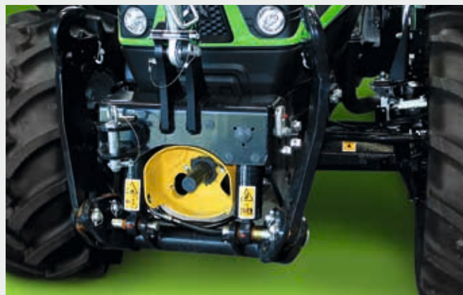
↑ A 2,100 kg capacity front power lift with a front power take-off @ 1,000 rpm is optional.
