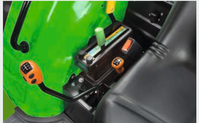
↑ To the right of the driver: gear lever, rear power lift and hydraulic control units ergonomically organised.
