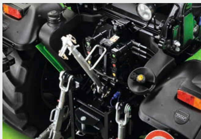
↑ The 55 l/min hydraulic pump supplies up to three rear control units.
