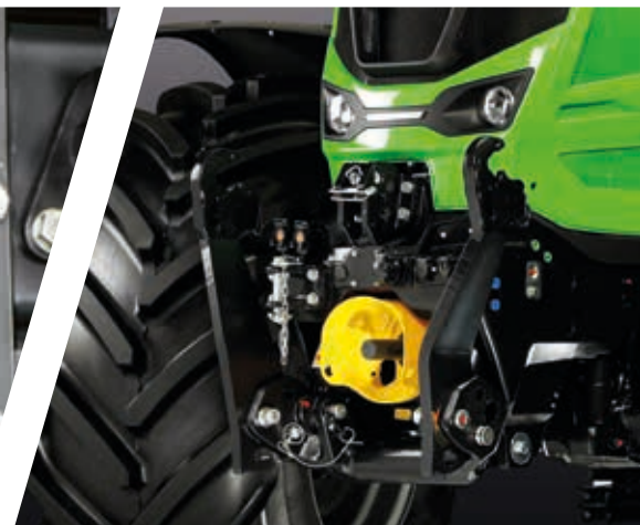
> 5450 kg lifting capacity and DualSpeed front PTO.
