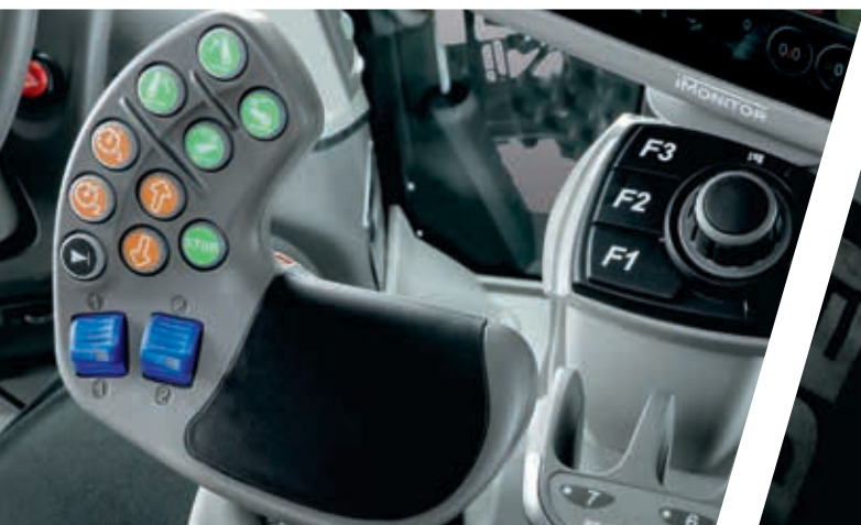
> Ergonomic joystick MaxCom.
