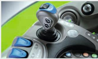
The redesigned armrest makes operation of the Series 7 even more relaxed and intuitive. All routine functions can be automated. Simply select the desired basic setting and reactivate at the press of finger. The new, highly ergonomic MaxCom joystick is used to control driving speed, direction of travel, Comfortip, and the linkages as well as for recalling cruise control speeds. Intuitive, without changing hand position or thinking long.
