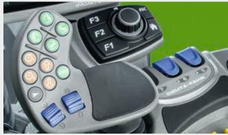
• Four driving speeds can be stored and recalled for optimising work processes.
