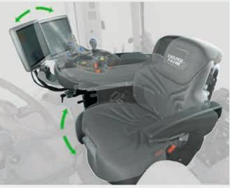
Seat with up to 20° rotation for added comfort and ease of operation.
