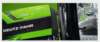
↑ Cab and bonnet are separated to reduce noise and vibration and increase comfort.
