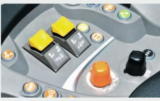
↑ The PTO activation and engagement (front/rear) is integrated into the armrest ...
