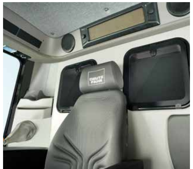
Dual grain tank inspection windows.
