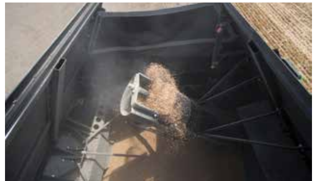
Large tank with 9500 ltr capacity extension on all models.
