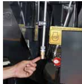
An air compressor is placed behind the radiators. The system has 3 outlets, one on each side and one on the engine compartment.
