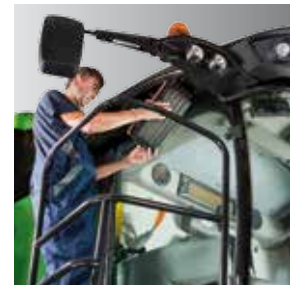
Cab filters in a convenient, low dust and easy to clean position.
