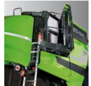
All radiators can be opened like a book and immediately accessed for periodic cleaning.
