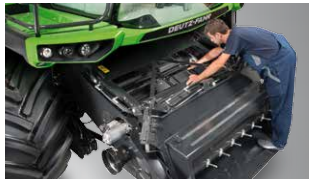
A wide opening panel provides access to the inside of the feeder housing for quick, easy and complete maintenance.
