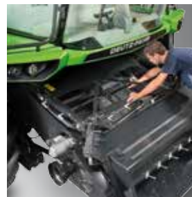
The feeder access cover plate, once removed, allows easy inspection and maintenance of the elevator chains and shafts.
