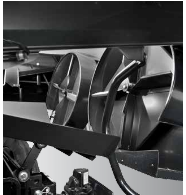
Chaff spreader with new conveyor and channels directing the chaff towards the 4-blade rotors.
