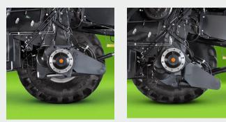
Both standard and Balance axle variants have a load capacity of 25 tonnes, for total peace of mind in even the most challenging conditions.
