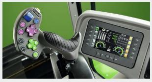
COMMANDER STICK. For controlling: 1) Position and inclination of header
