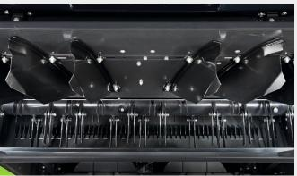
Straw Chopper, for even more effective material distribution, the straw chopper may also be equipped with deflectors, adjusted electrically from the cab, to adjust spreading to weather conditions.
