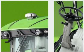
Easy installation of the precision farming systems, full integration of the electrical steering, the GPS antenna, the yield sensors and the Isobus ECU.
