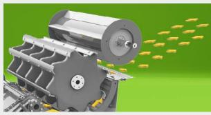
THRESHING DRUM, CONCAVE AND STRAW BEATER. A broad 600 mm diameter threshing drum measuring 1.27 m in width for the 5 straw walker model and 1.52 m in width for the 6 straw walker model, and a multi-segment concave with a pitch of 121° ensure perfect threshing results in all conditions.
