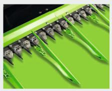
The offset configuration of the knife sections reduce wear and ensures excellent cutting results in all conditions.
