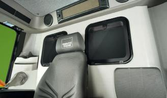
Visaual grain tank monitoring. A double window in the cab lets the operator visually check the fill level of the tank and the quality of the grain harvested.
