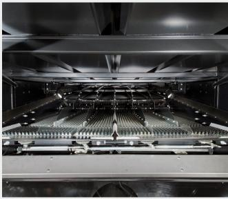
An (optional) electrically operated sieve adjustment system lets the operator adjust sieve clearance instantaneously in relation to harvesting conditions.
