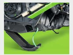
The sensor skids allow the header to follow the contours of the terrain precisely and make instant adjustments to ensure an even cutting height.
