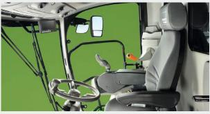
Ergonomic seat with mechanical or pneumatic adjustment and adjustable steering column for setting a comfortable driving position.
