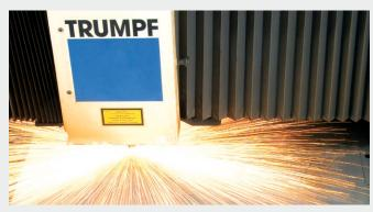
Every part of the combine structure is produced with the use of Laser cutting machines which, starting from the 3D drawing, allow the finished piece to be made.
