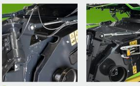
Adjustable cutting angle for following the contours of uneven terrain perfectly.
