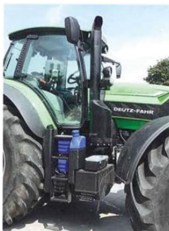
The diesel tank holds 435 l, the AdBlue tank 50 l. It can only be filled from the right.
