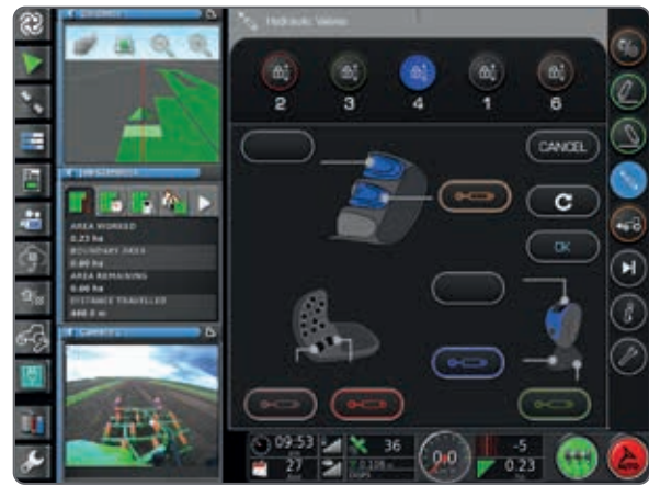
Spool valves - The order of spool valves can be changed, as well as flow rate and time control.
