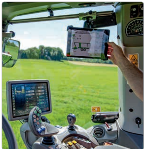
With the installed tablet inside the cab guidance can be displayed or ISOBUS UT operated.
