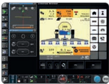
Independent of application profile – all ISOBUS implements are displayed through the Universal Terminal of the iMonitor.
