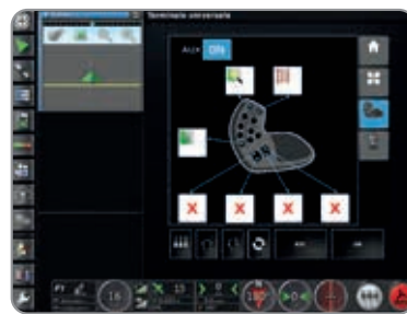
AUX-N assignment: depending on features, up to 10 functions can be assigned on the armrest and 9 additional functions in the monitor.
